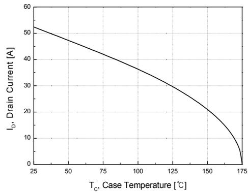
**Figure 10. Maximum Drain Current vs. Case Temperature**
