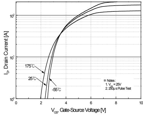
**Figure 2. Transfer Characteristics**
