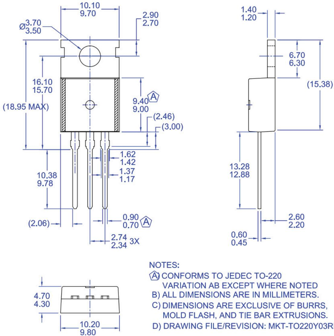
**Figure 16. TO220, Molded, 3-Lead, Jedec Variation AB**
