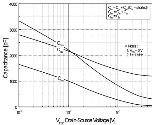
**Figure 5. Capacitance Characteristics**
