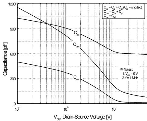
Figure 5. Capacitance Characteristics
