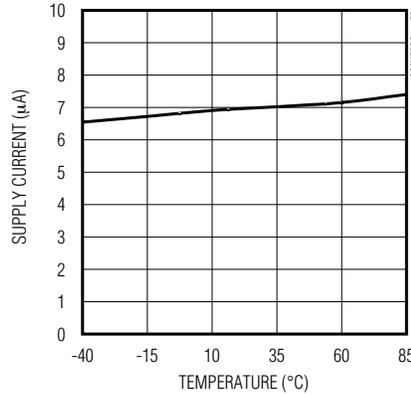
**SHUTDOWN SUPPLY CURRENT vs. TEMPERATURE (MAX5531)**
