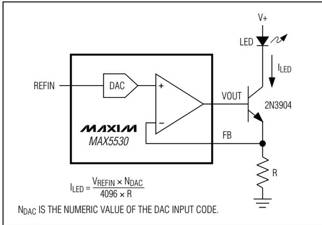
Figure 4. Programmable Current Source Driving an LED
