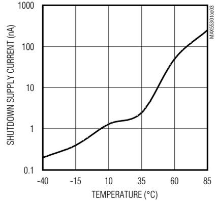
**STANDBY SUPPLY CURRENT vs. TEMPERATURE (MAX5531)**
