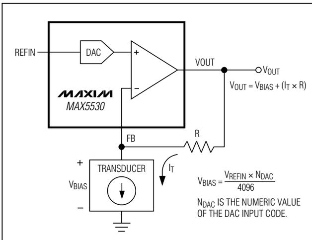
Figure 5. Transimpedance Configuration for a Voltage-Biased Current-Output Transducer
