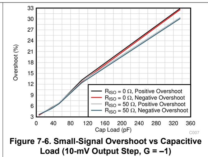
Figure 7-6. Small-Signal Overshoot vs Capacitive Load (10-mV Output Step,  $G = -1$ )
