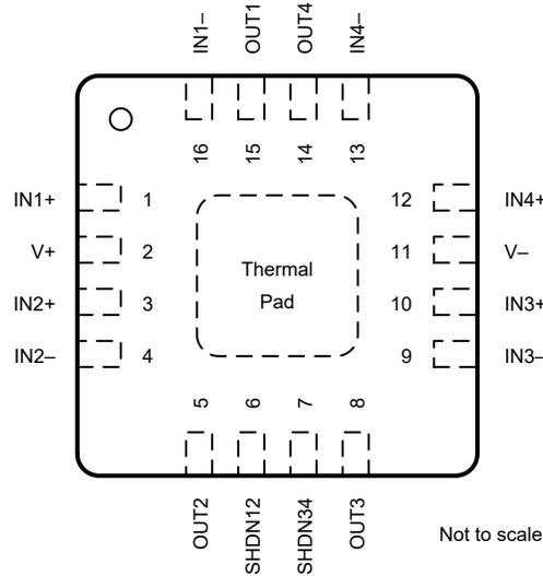
A. Connect thermal pad to V-. See [Packages with an Exposed Thermal Pad](#) section for more information.
