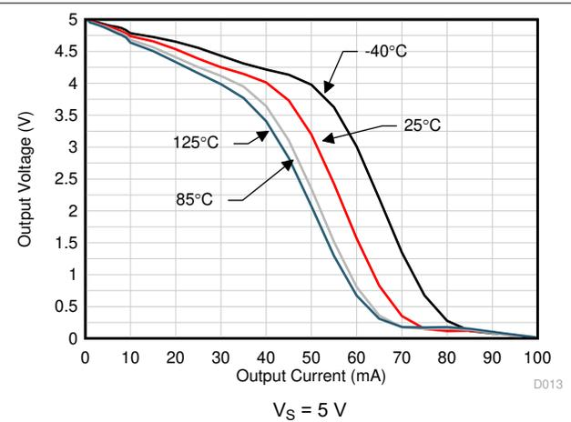
Figure 6-16. Output Voltage Swing vs Output Current (Sourcing)
