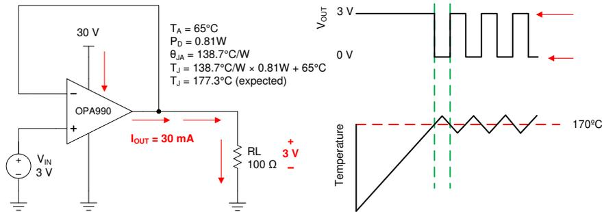
Figure 7-4. Thermal Protection
