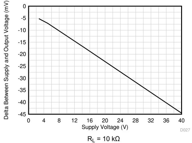
**Figure 6-32. Output Swing vs Supply Voltage, Negative Swing**
