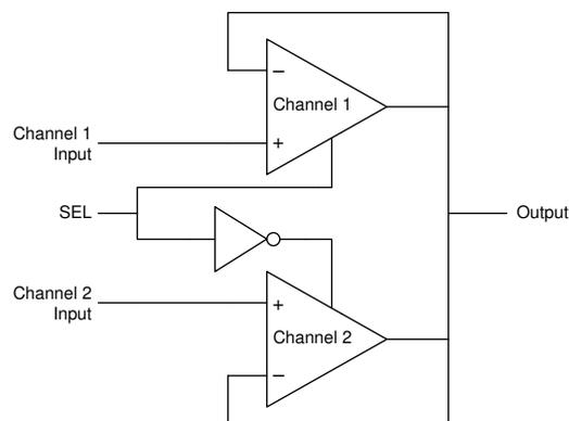
Figure 8-1. High Voltage Buffered Multiplexer
