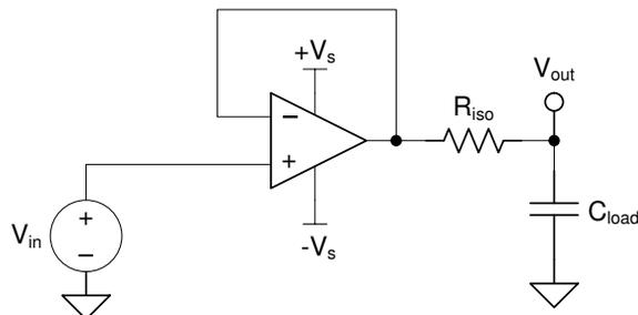
Figure 7-7. Extending Capacitive Load Drive With the OPA990
