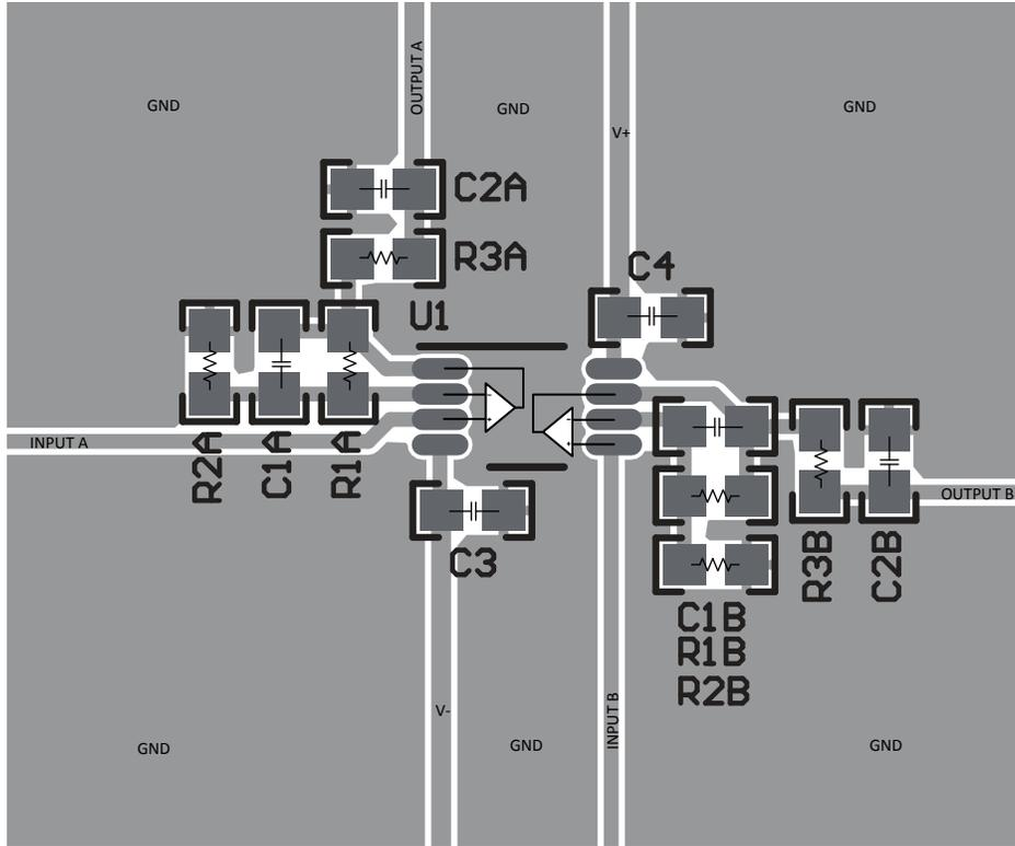
Figure 10-4. Example Layout for VSSOP-8 (DGK) Package
