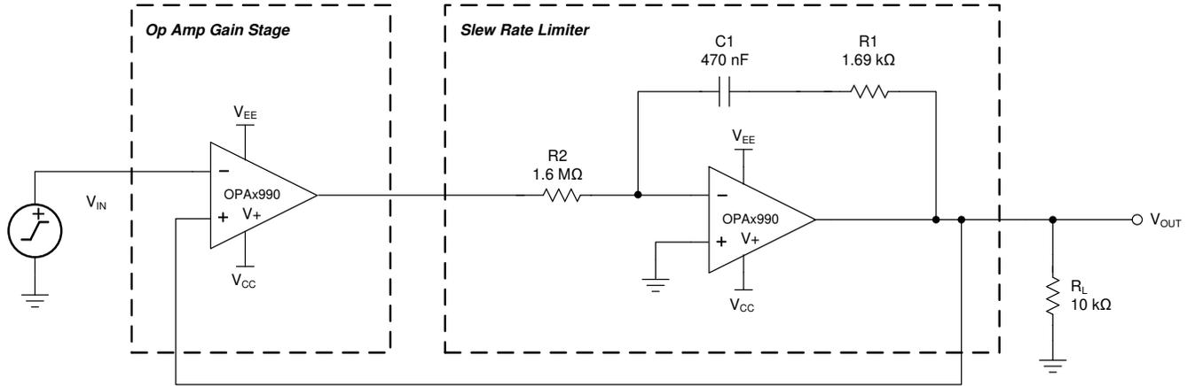
**Figure 8-2. Slew Rate Limiter Uses One Op Amp**
