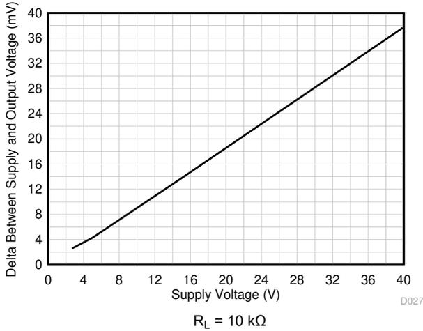
**Figure 6-31. Output Swing vs Supply Voltage, Positive Swing**
