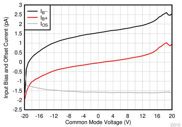
**Figure 6-12. Input Bias Current vs Common-Mode Voltage**
