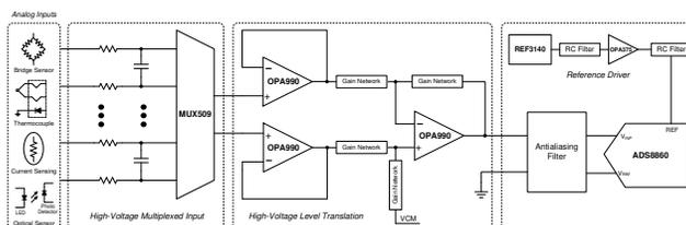
**OPAx990 in a High-Voltage, Multiplexed, Data-Acquisition System**
