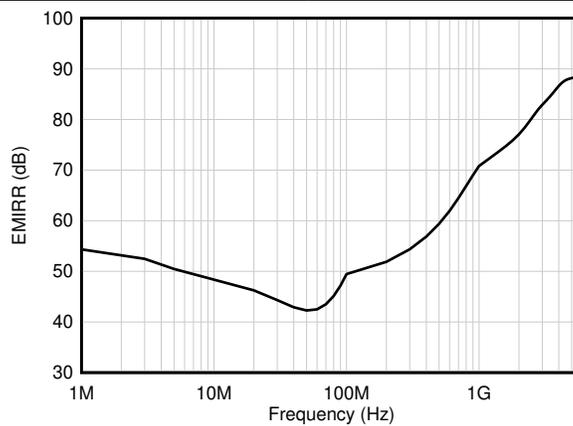
**Figure 6-47. EMIRR (Electromagnetic Interference Rejection Ratio) vs Frequency**
