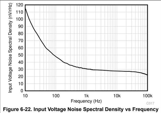
**Figure 6-22. Input Voltage Noise Spectral Density vs Frequency**
