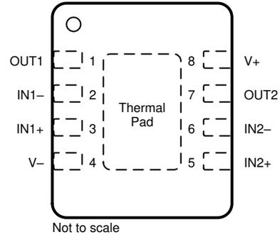
A. Connect thermal pad to V-. See [Packages with an Exposed Thermal Pad](#) section for more information.
