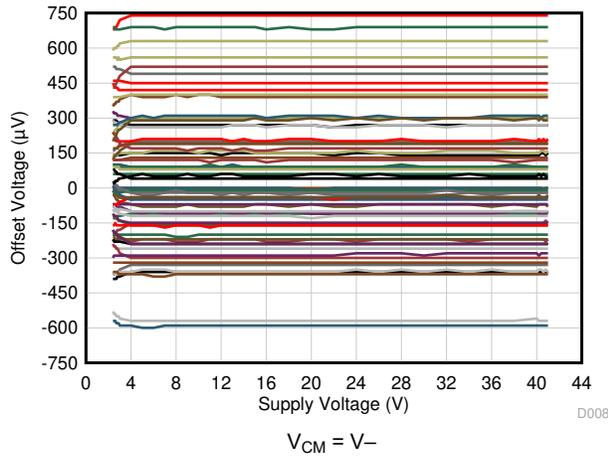
**Figure 6-9. Offset Voltage vs Power Supply**
