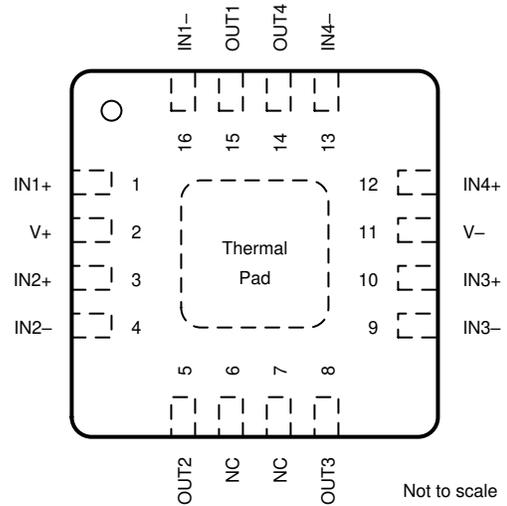
A. Connect thermal pad to V-. See [Packages with an Exposed Thermal Pad](#) section for more information.
