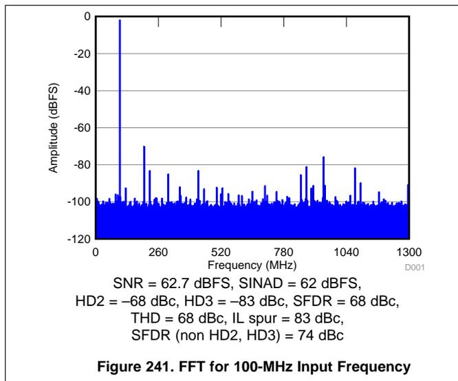
Figure 241. FFT for 100-MHz Input Frequency
