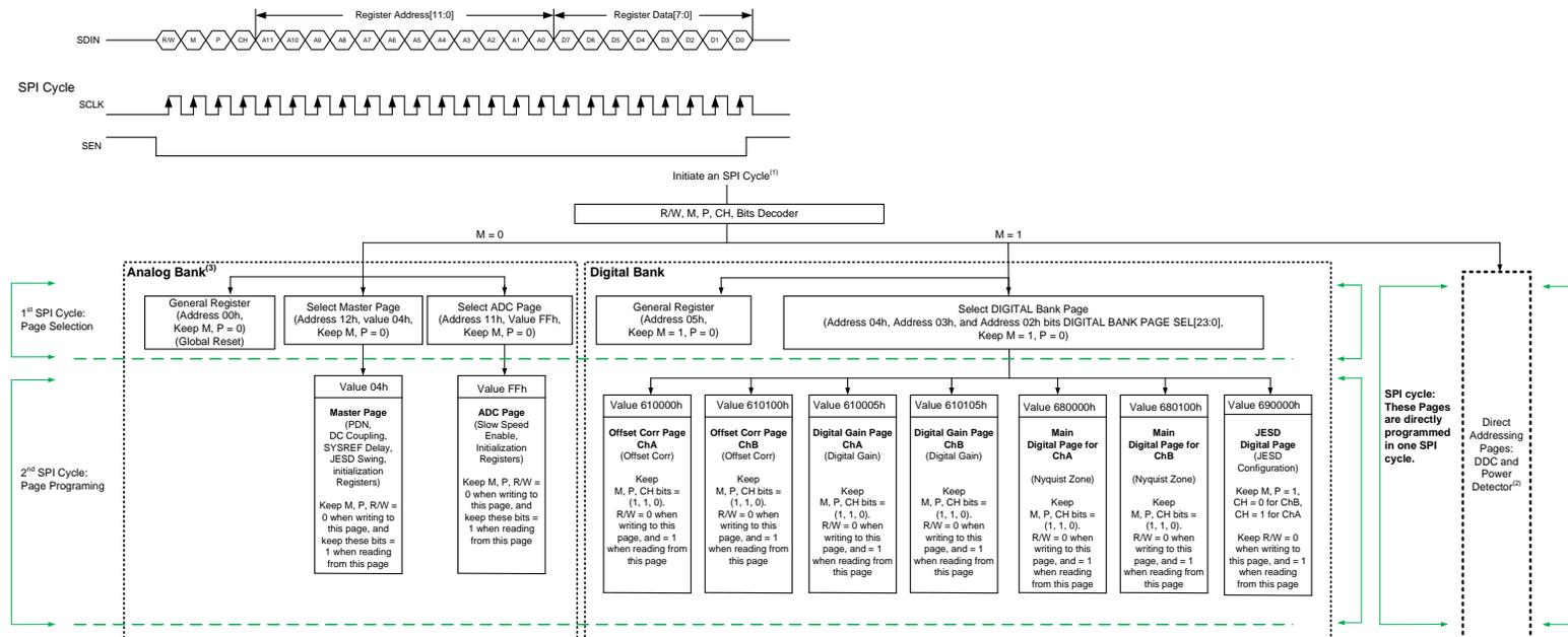
In general, SPI writes are completed in two steps. The first step is to access the necessary page. The second step is to program the desired register in that page. When a page is accessed, the registers in that page can be programmed multiple times.
