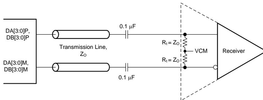
Figure 100. External Serial JESD204B Interface Connection
