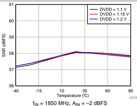
Figure 25. Signal-to-Noise Ratio vs DVDD Supply and Temperature
