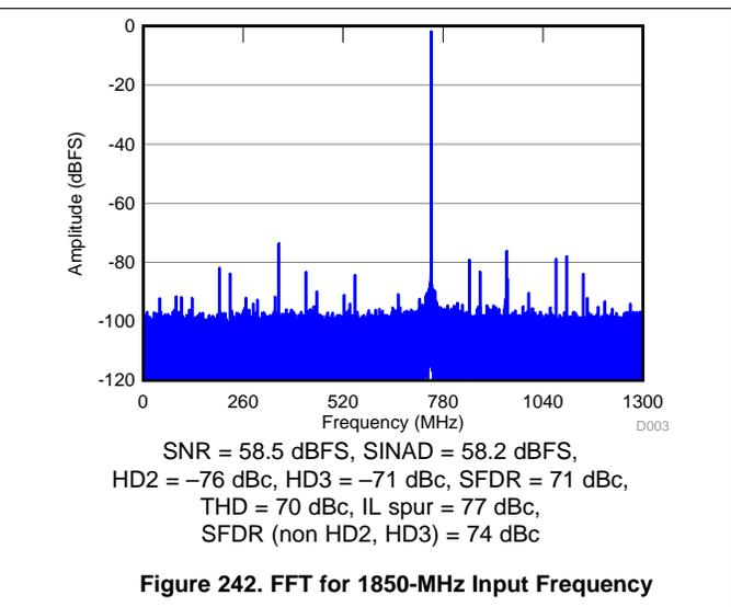
Figure 242. FFT for 1850-MHz Input Frequency
