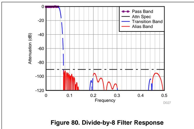
Figure 80. Divide-by-8 Filter Response
