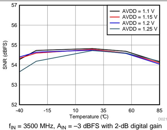
Figure 23. Signal-to-Noise Ratio vs AVDD Supply and Temperature
