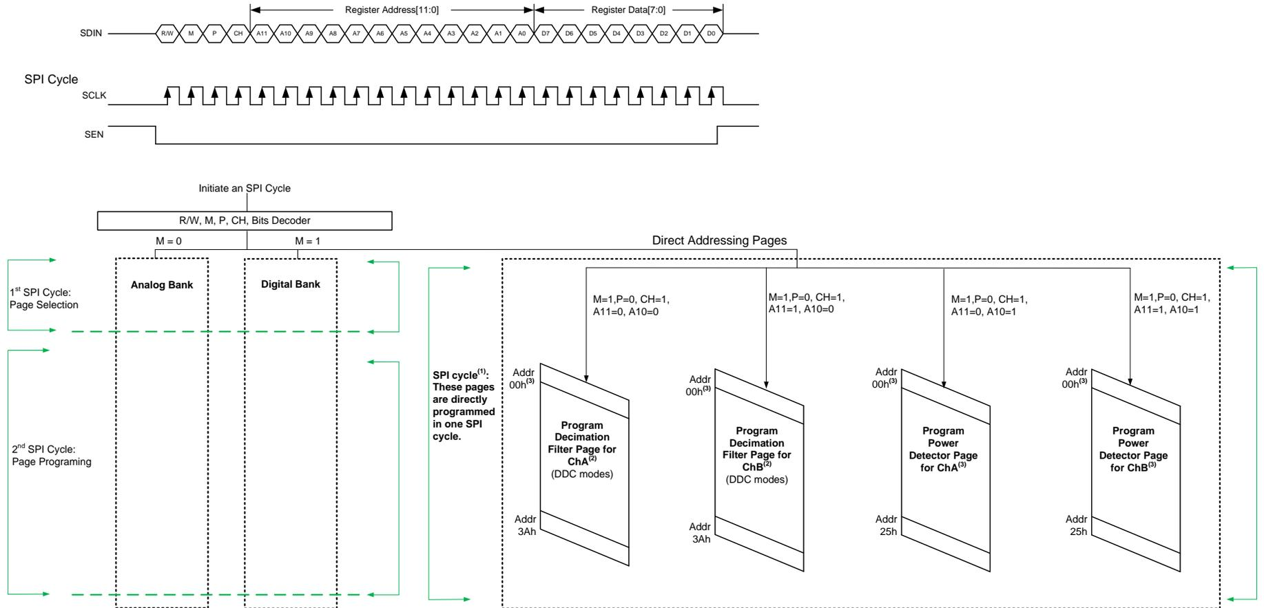
Registers in the decimation filter page and the power detector page can be directly programmed in one SPI cycle.
