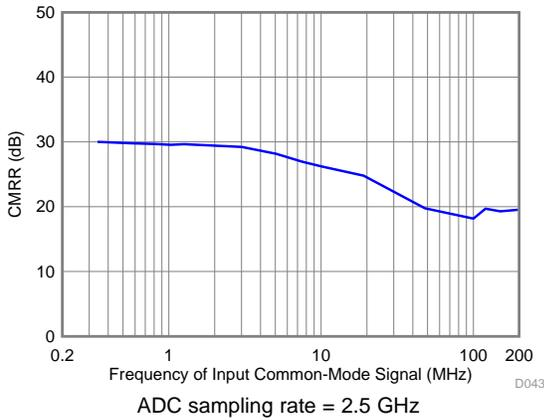
**Figure 45. Common-Mode Rejection Ratio vs Signal Frequency**
