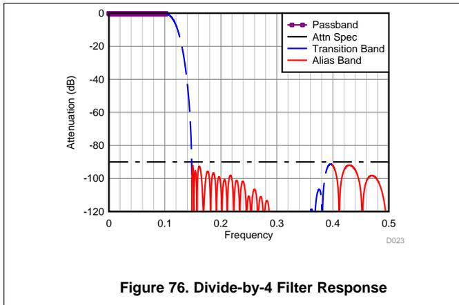
Figure 76. Divide-by-4 Filter Response
