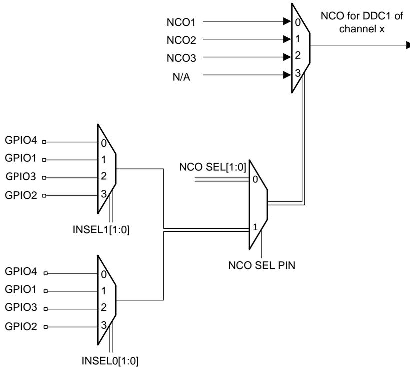
Figure 99. NCO Switching from GPIO and SPI
