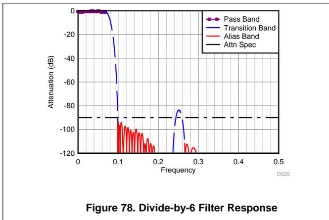
Figure 78. Divide-by-6 Filter Response
