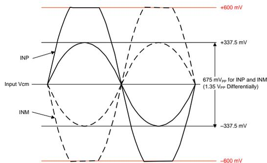
Figure 64. Clamp Response Timing Diagram
