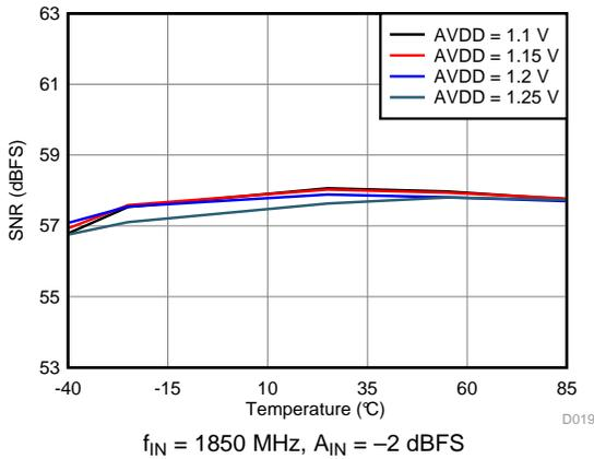
Figure 21. Signal-to-Noise Ratio vs AVDD Supply and Temperature
