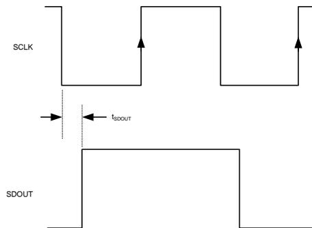
**Figure 114. SDOUT Timing**
