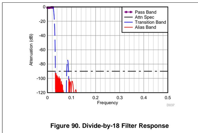
Figure 90. Divide-by-18 Filter Response
