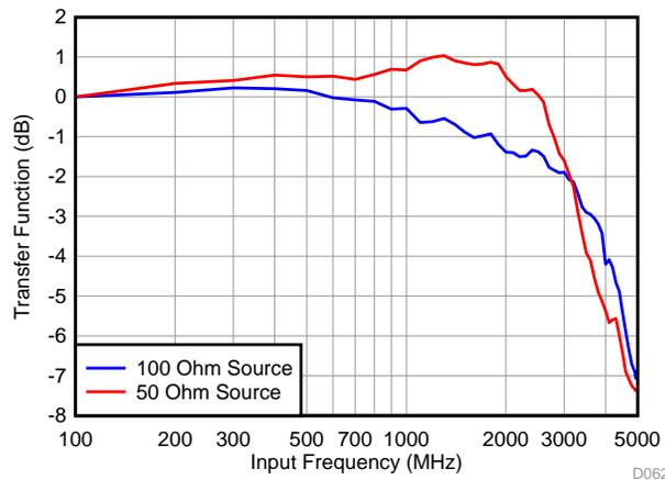
Figure 62. Input Bandwidth with a 100-Ω Source Resistance
