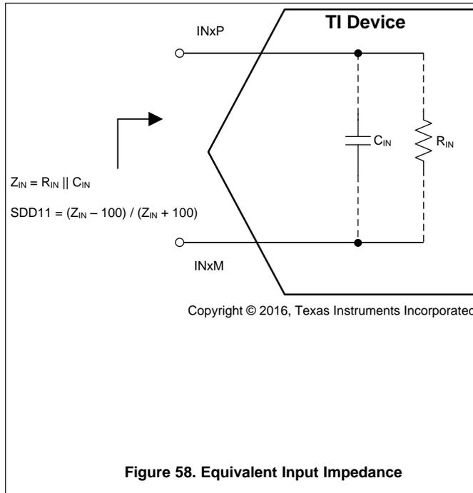
Figure 58. Equivalent Input Impedance
