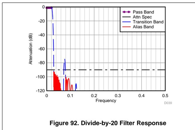
Figure 92. Divide-by-20 Filter Response
