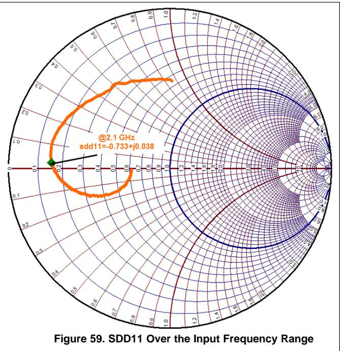
Figure 59. SDD11 Over the Input Frequency Range
