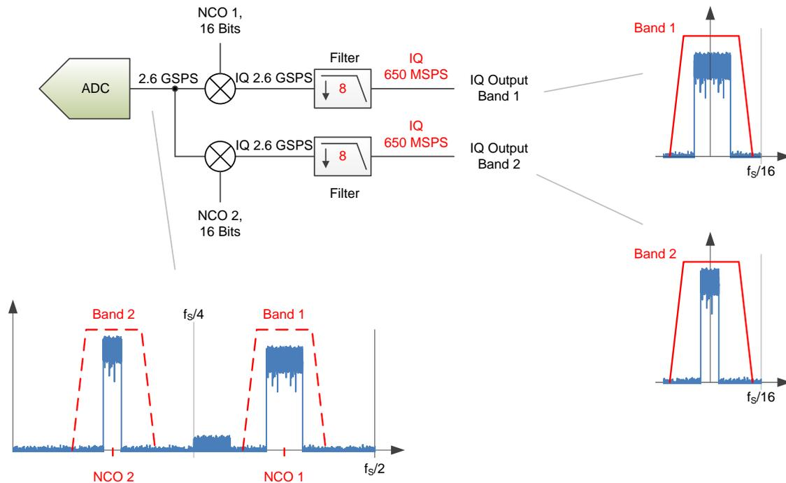
Figure 74. Dual-Band Example
