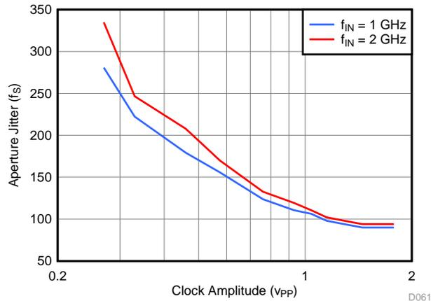
Figure 66. Equivalent Aperture Jitter vs Input Clock Amplitude
