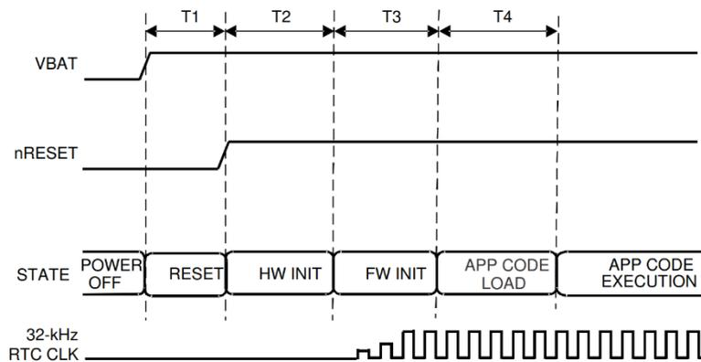
**Figure 4-3. First-Time Power-Up and Reset Removal Timing Diagram**
