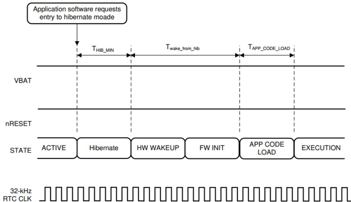
**Figure 4-4. Wake Up From Hibernate Timing Diagram**
