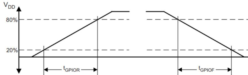
**Figure 4-9. GPIO Timing Diagram**
