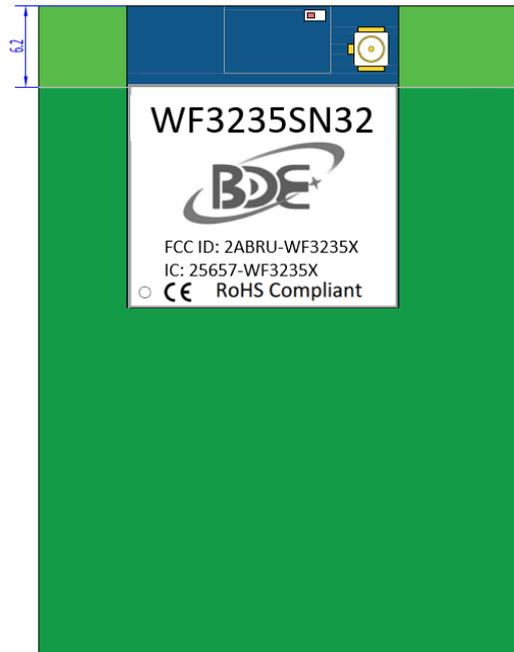
**Figure 6-3. BDE-WF3235 Layout Guidelines**
