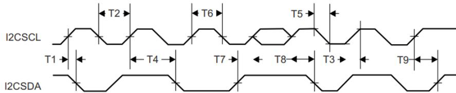
**Figure 4-10. I<sup>2</sup>C Timing Diagram**
