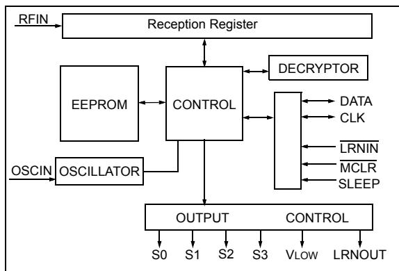
The Manufacturer's Code, transmitter keys, and synchronization information are stored in protected on-chip EEPROM. The HCS512 uses the DATA and CLK inputs to load the Manufacturer's Code which cannot be read out of the device.
