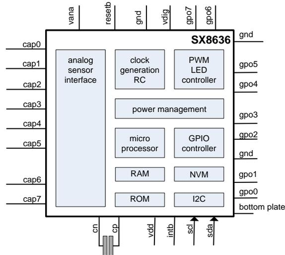
Figure 3 Simplified block diagram of the SX8636
