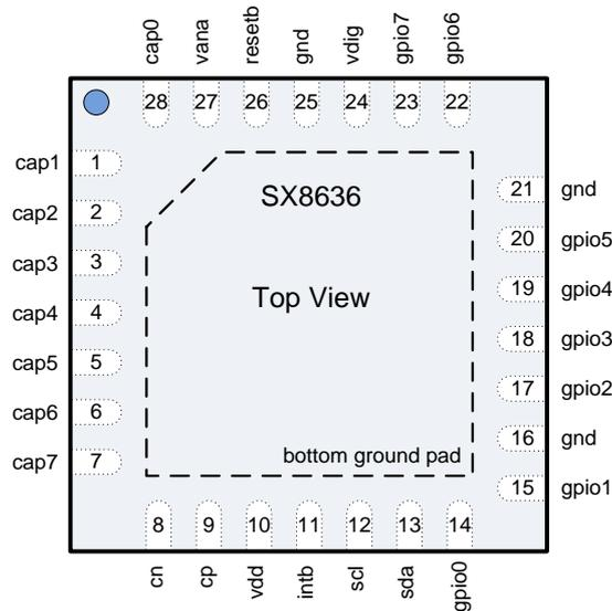
Figure 1 Pinout Diagram
