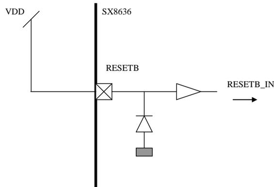
*Figure 36 Simplified diagram of RESETB without host control*
