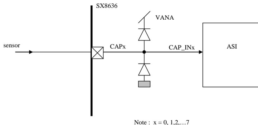
*Figure 30 Simplified diagram of CAP0, CAP1, ..., CAP7*
