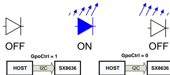
*Figure 24 LED Control in GPO mode, Autolight OFF*
