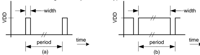
Figure 22 PWM definition, (a) small pulse width, (b) large pulse width
