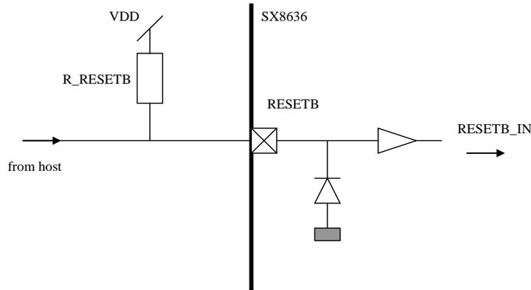
*Figure 35 Simplified diagram of RESETB controlled by host*
