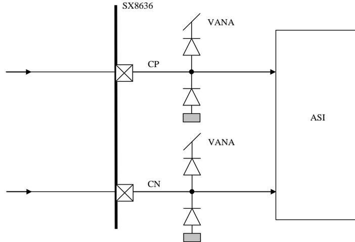
Figure 31 Simplified diagram of CN and CP
