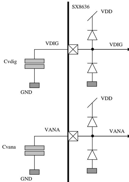
Figure 39 Simplified diagram of VANA and VDIG
