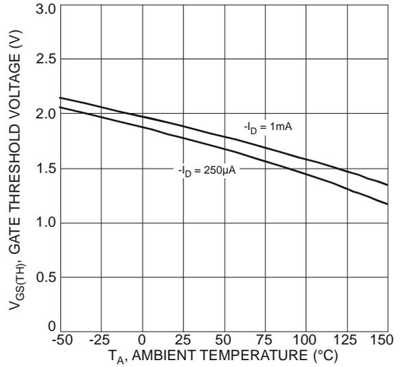
Figure 8 Gate Threshold Variation vs. Ambient Temperature
