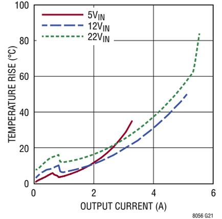
Temperature Rise vs Output Current (8V<sub>OUT</sub>)
