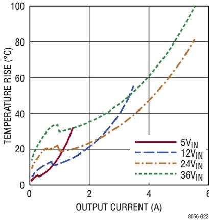
Temperature Rise vs Output Current (18V<sub>OUT</sub>)
