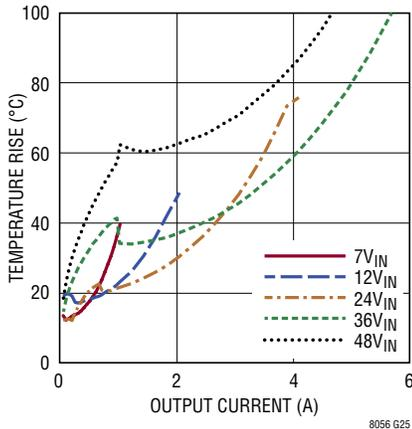
Temperature Rise vs Output Current (36V<sub>OUT</sub>)
