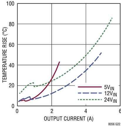
Temperature Rise vs Output Current (12V<sub>OUT</sub>)
