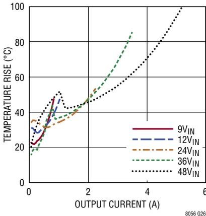
Temperature Rise vs Output Current (48V<sub>OUT</sub>)
