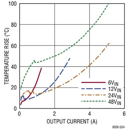
Temperature Rise vs Output Current (24V<sub>OUT</sub>)
