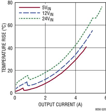
Temperature Rise vs Output Current (5V<sub>OUT</sub>)
