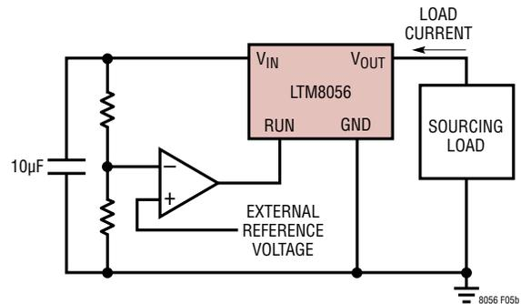
**Figure 5b. This Comparator Circuit Turns Off the LTM8056 if the Input Rises Above a Predetermined Threshold. When the LTM8056 Turns Off, the Energy Stored in the Internal Inductor Will Raise  $V_{IN}$  a Small Amount Above the Threshold**
