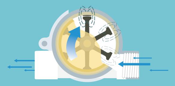
This flow meter is intended for medium-to-high flow ranges from 5.7 L/min (1.5GPM) up to 75.70 L/min (20 GPM).
