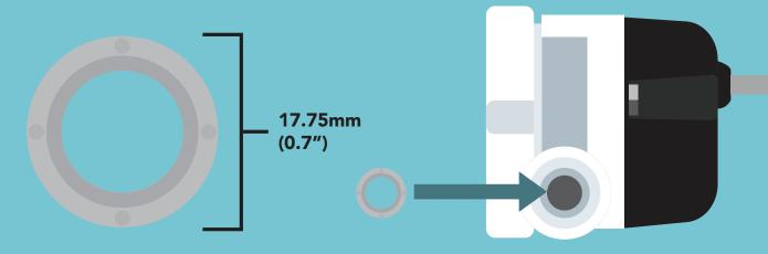
A low flow adapter is included with the Atlas Scientific 1/2" Flow Meter.
