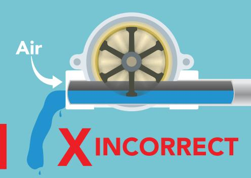
FOR ACCURATE READINGS, YOU CANNOT HAVE AIR IN THE LINE.
