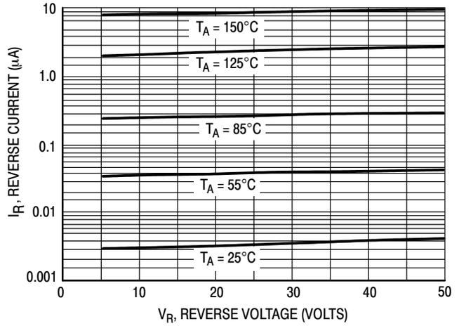
**Figure 3. Leakage Current**
