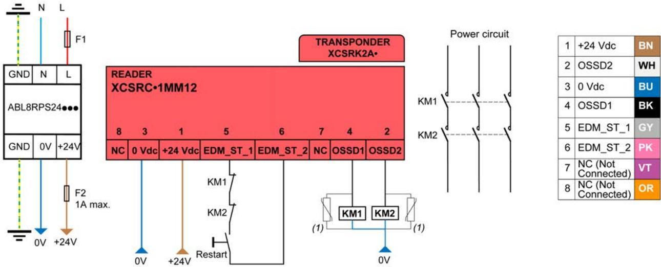
(1) Use of arc suppressors for KM1 & KM2 is recommended.
