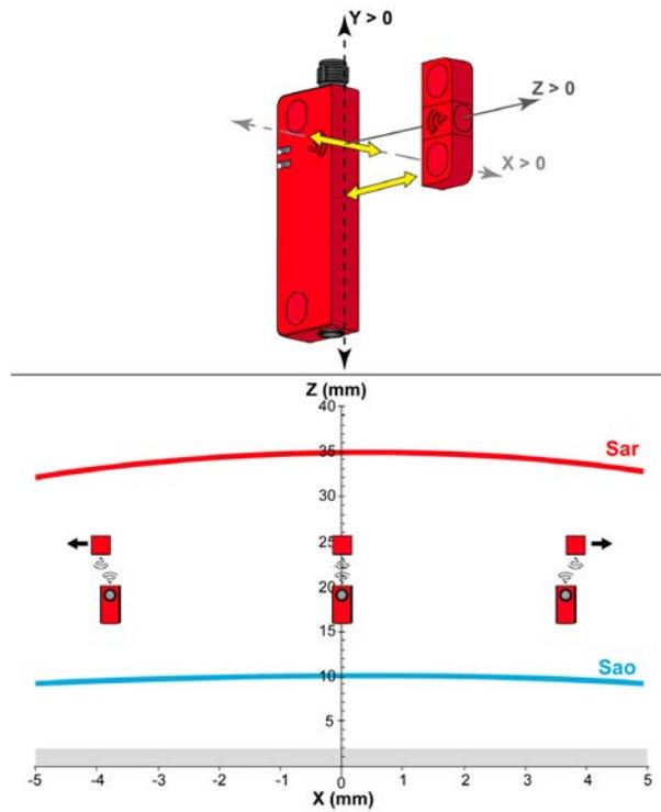
Typical switch-on and switch-off sensing distances along Y axis as function of Z. (longitudinal misalignment for X=0)
