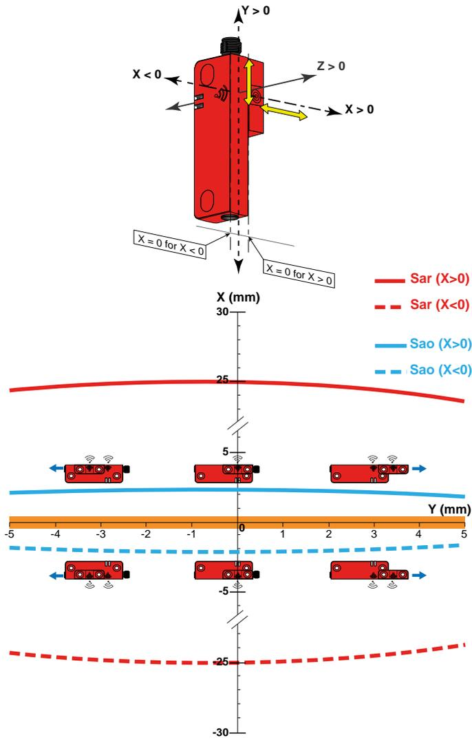
Figure of  $S_{ao}$  and  $S_{ar}$  sensing distances along Z axis as function of X (transverse misalignment for Y=0)
