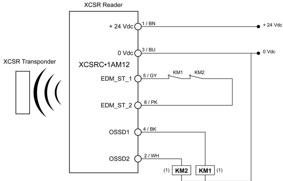
(1) Use of arc suppressors for KM1 & KM2 is recommended.
