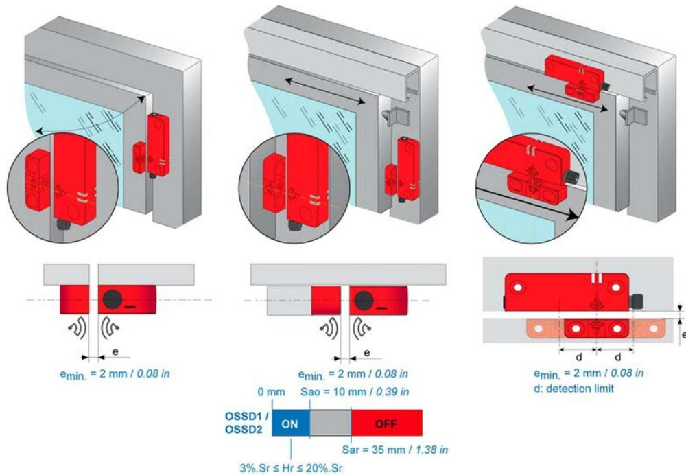
e Recommended minimum mounting distance between transponder and reader.
