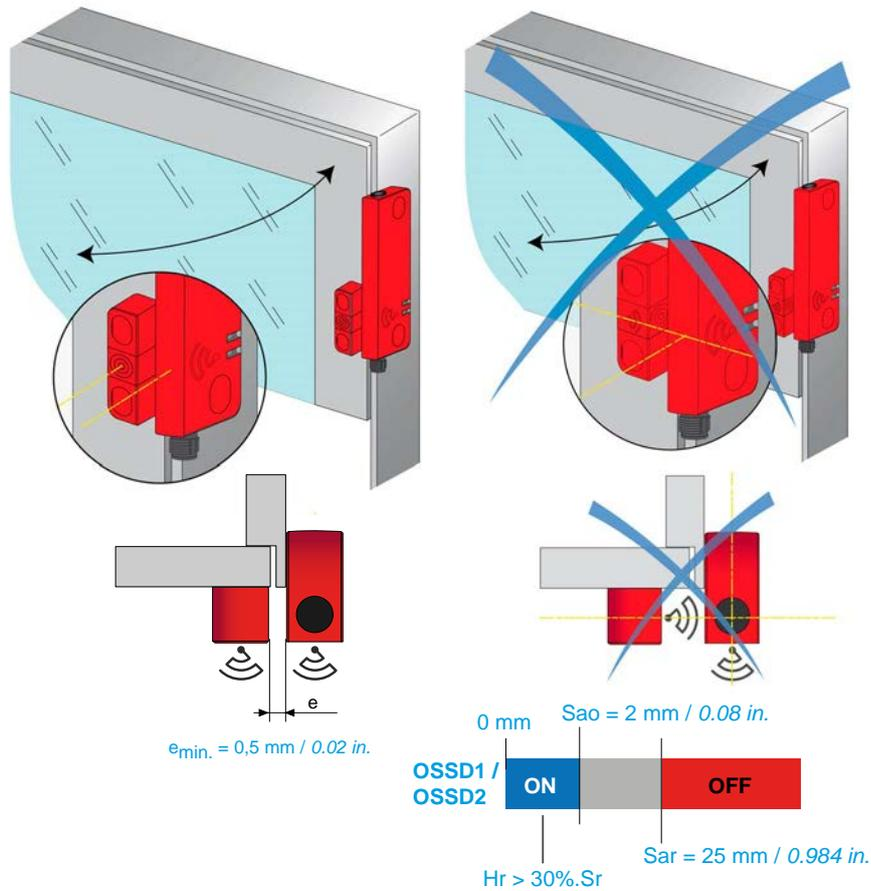
**e** Recommended minimum mounting distance between transponder and reader.
