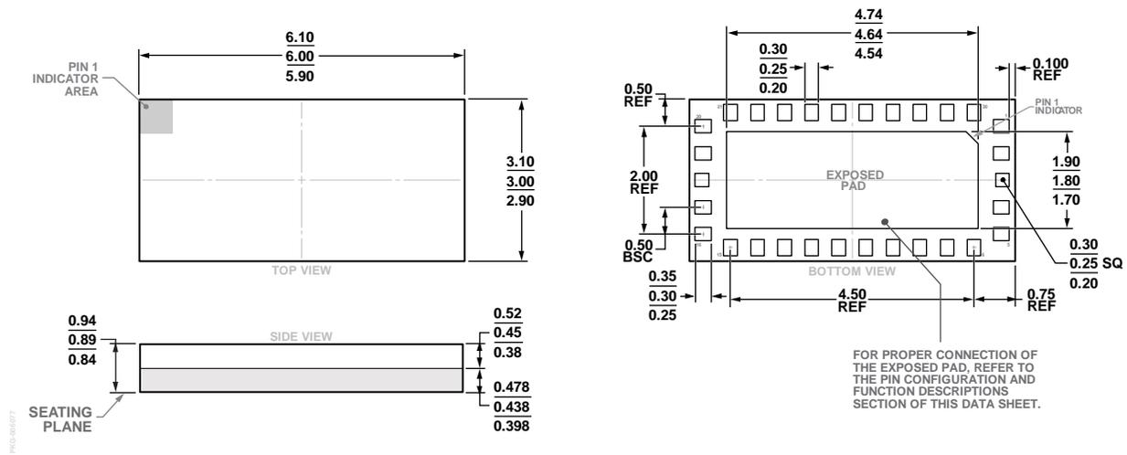
Figure 21. 30-Terminal Land Grid Array Package [LGA] (CC-30-4)
