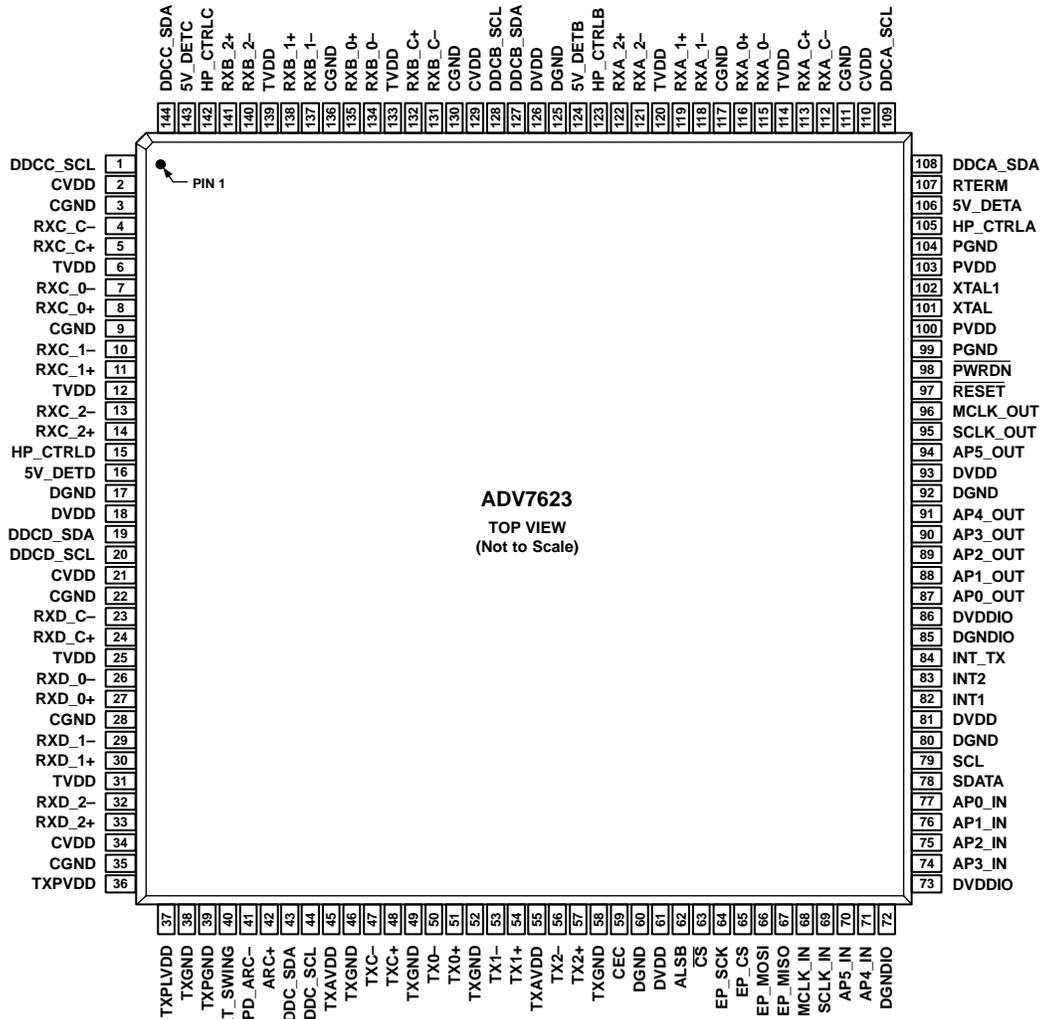
Figure 5. Pin Configuration
