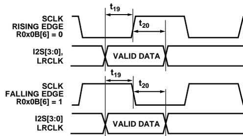
Figure 4. I<sup>2</sup>S Input Timing
