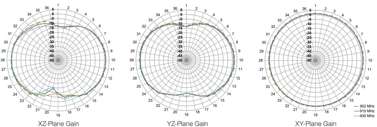
Figure 9. Radiation Patterns for ANT-8/9-IPW1-SMA, Edge Bent
