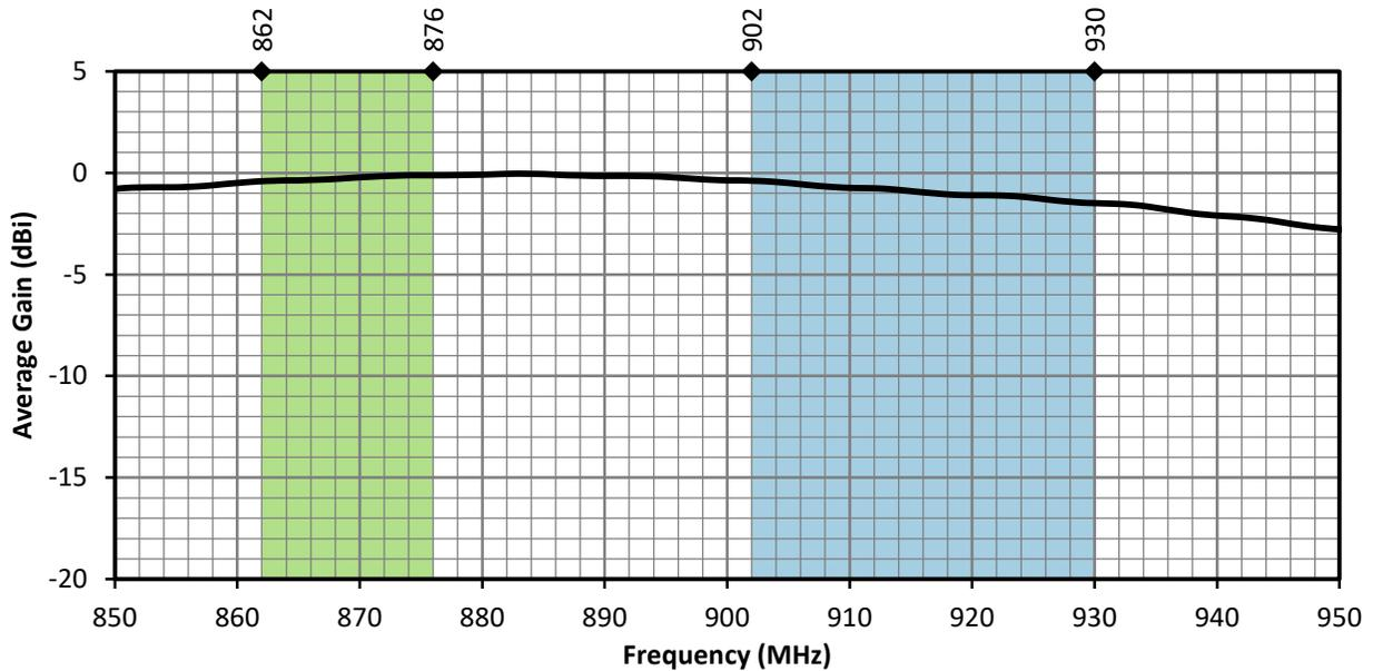
Figure 7. ANT-8/9-IPW1-SMA Antenna Average Gain, Edge Bent
