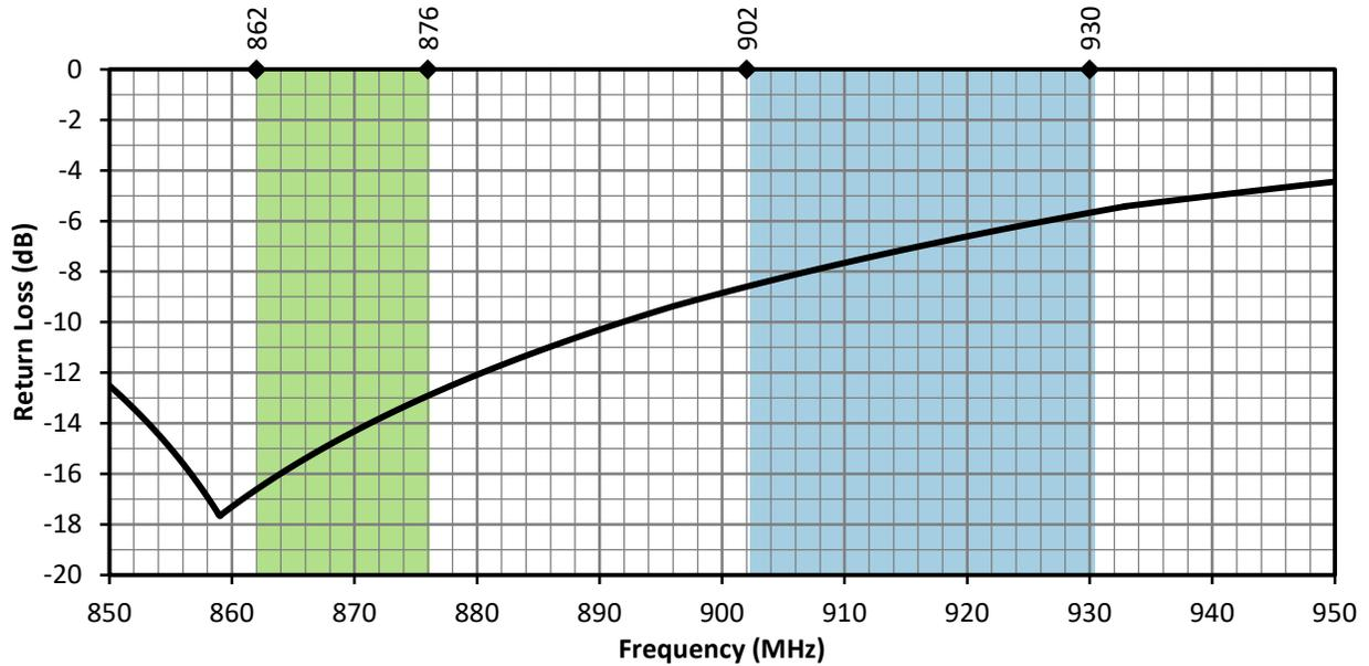
Figure 5. ANT-8/9-IPW1-SMA Antenna Return Loss, Edge Bent
