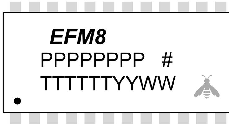
Figure 8.3. QSOP24 Package Marking
