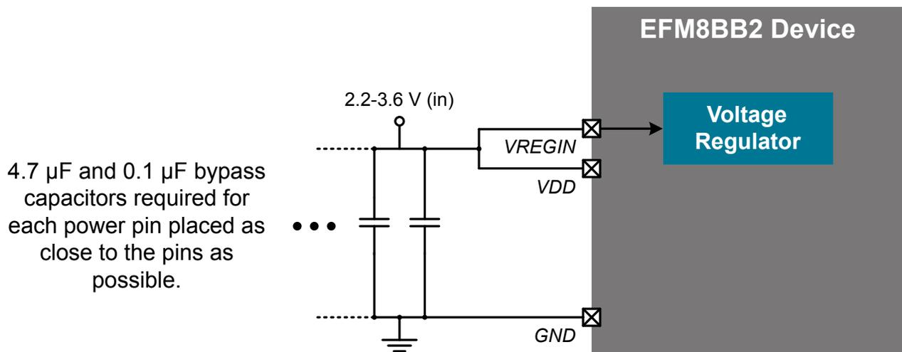
Figure 5.2. Connection Diagram with Voltage Regulator Not Used
