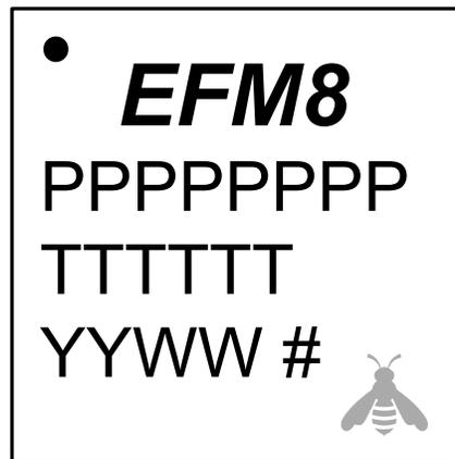
Figure 7.3. QFN28 Package Marking
