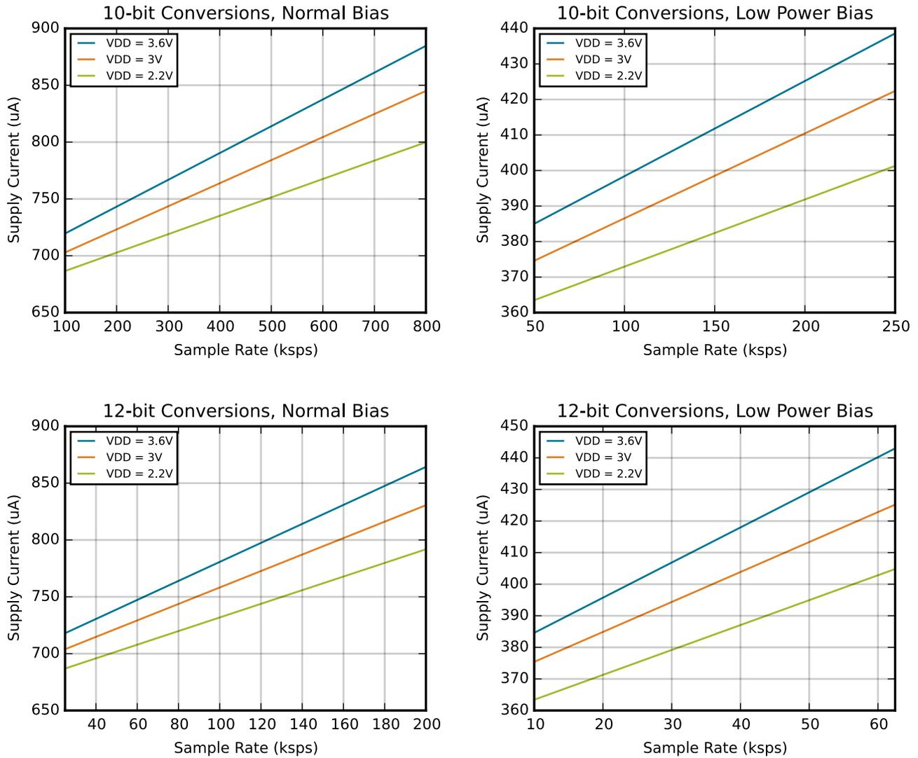
Figure 4.5. Typical ADC0 Supply Current in Normal (always-on) Mode
