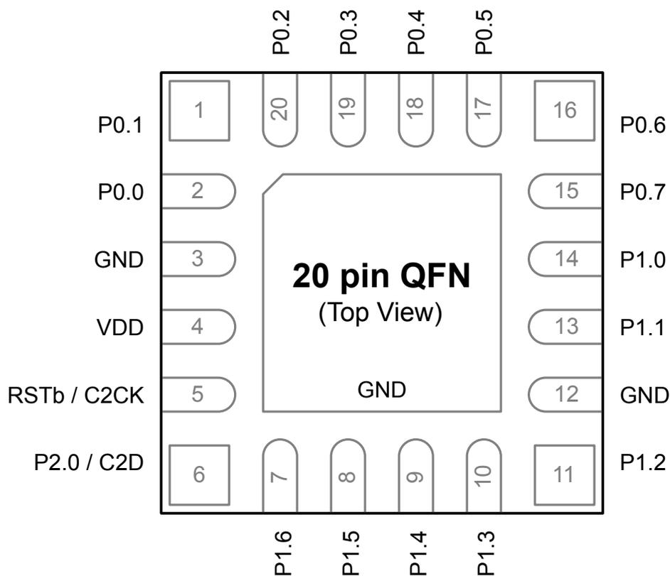
Figure 6.3. EFM8BB2x-QFN20 Pinout
