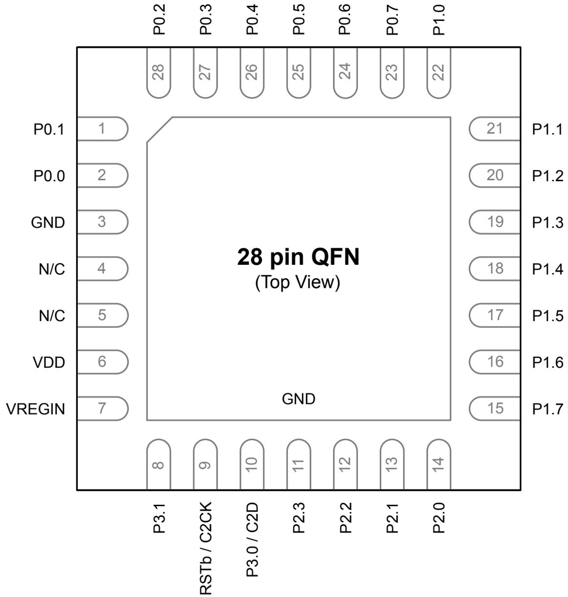
Figure 6.1. EFM8BB2x-QFN28 Pinout
