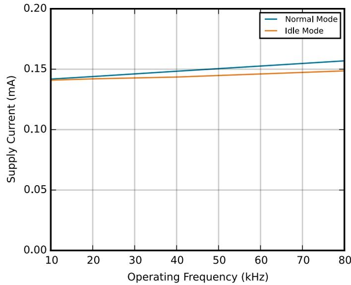
Figure 4.3. Typical Operating Supply Current using LFOSC
