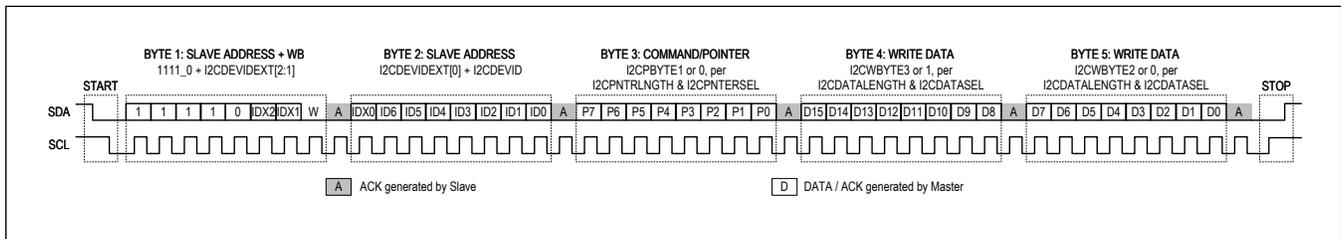
Figure 77. I<sup>2</sup>C Write Mode Transaction Example -- 10-Bit Address, I2C10BIT = 1
