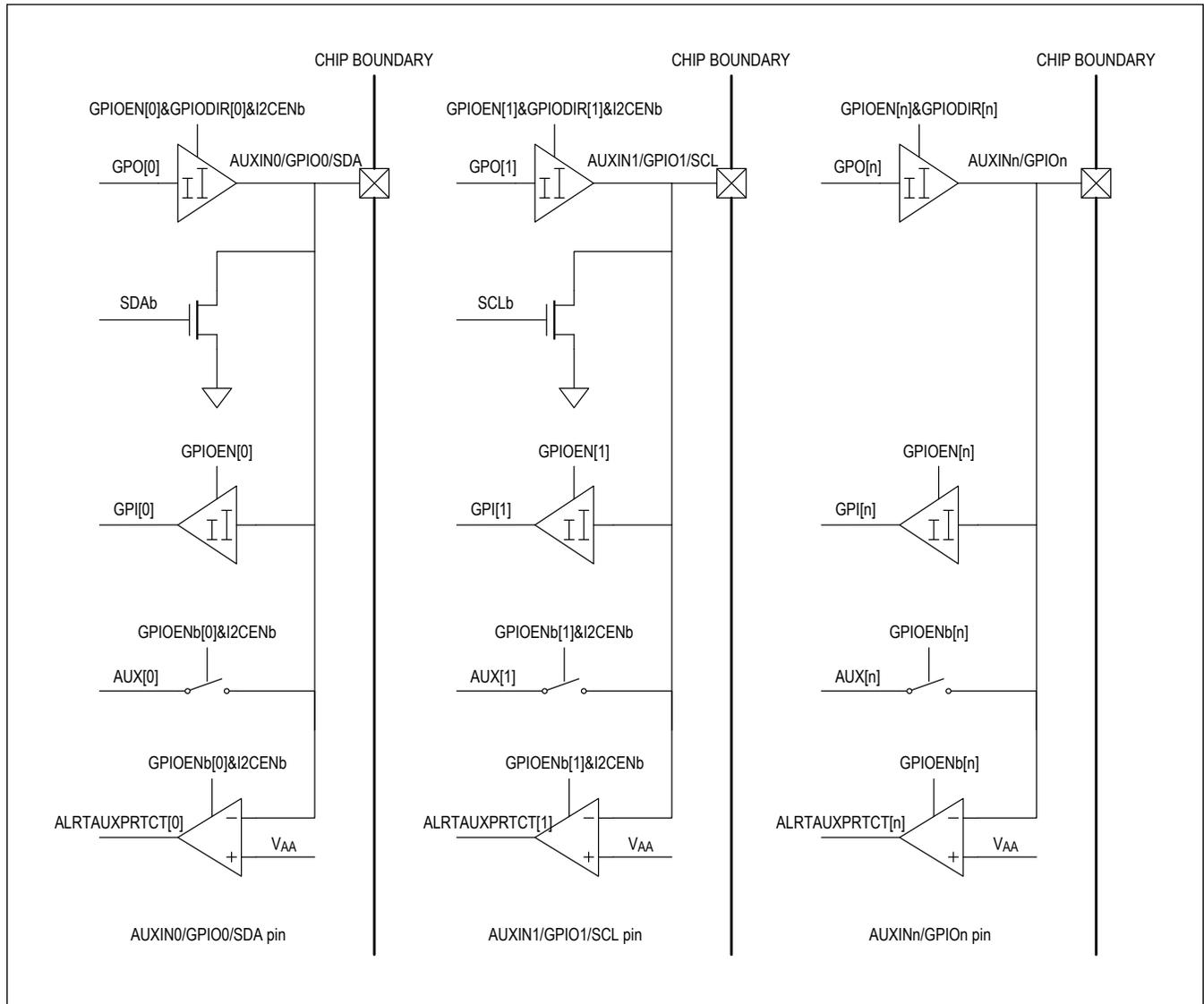
Figure 11. AUX/GPIO/I<sup>2</sup>C Pin Connections
