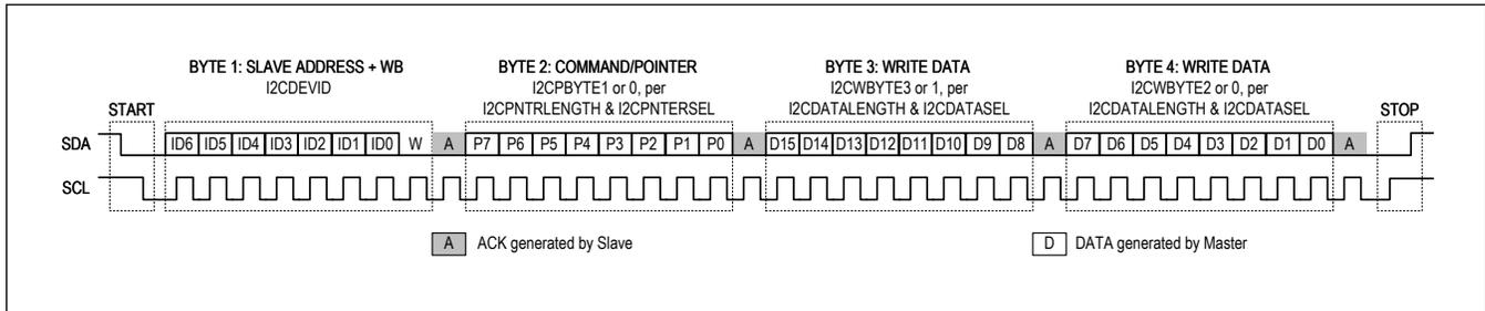
Figure 76. I<sup>2</sup>C Write Mode Transaction Example -- 7-Bit Address, I2C10BIT = 0
