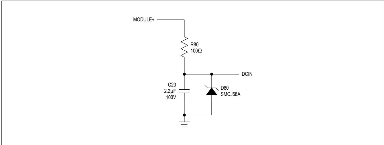
Figure 116. Power-Supply Connection
