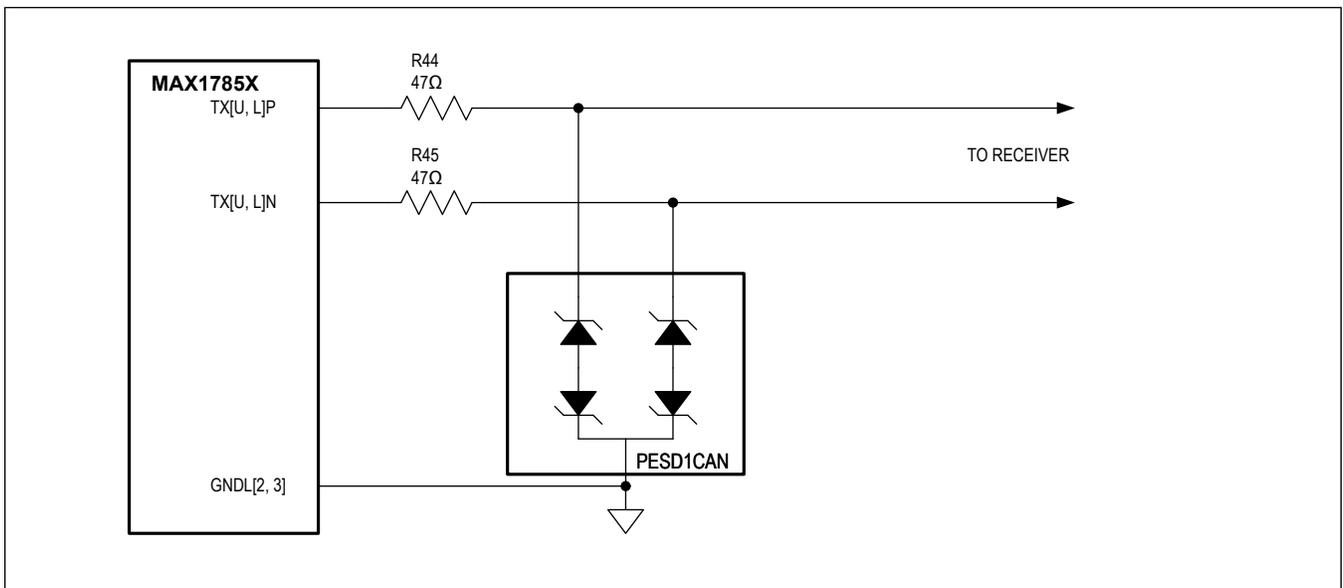
Figure 121. External ESD Protection for UART TX Ports
