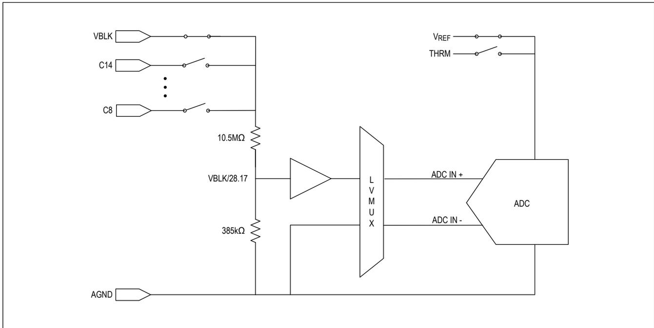
Figure 8. Block-Measurement Path
