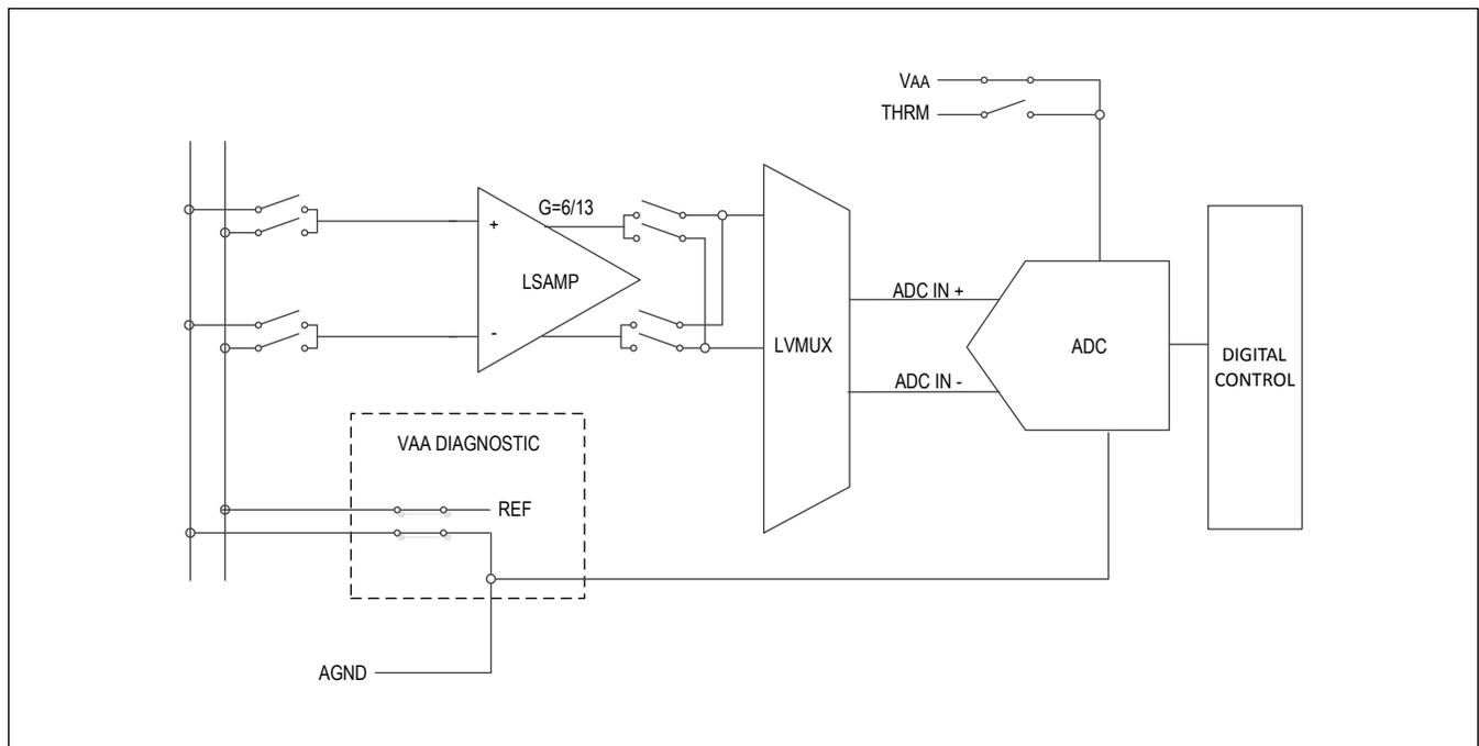
Figure 90.  $V_{AA}$  Diagnostic
