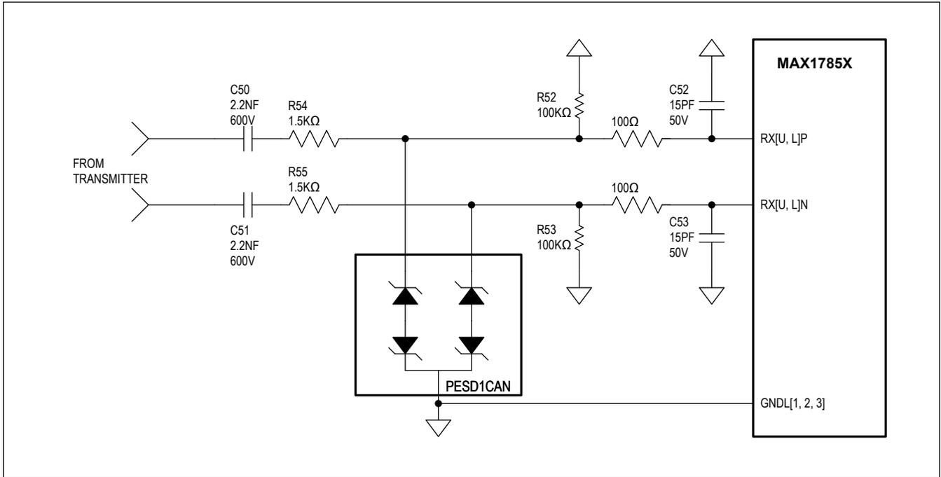
Figure 122. External ESD Protection for UART RX Ports
