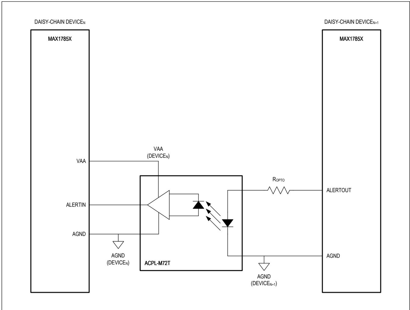
Figure 128. Single-End ALERT Interface in UART mode
