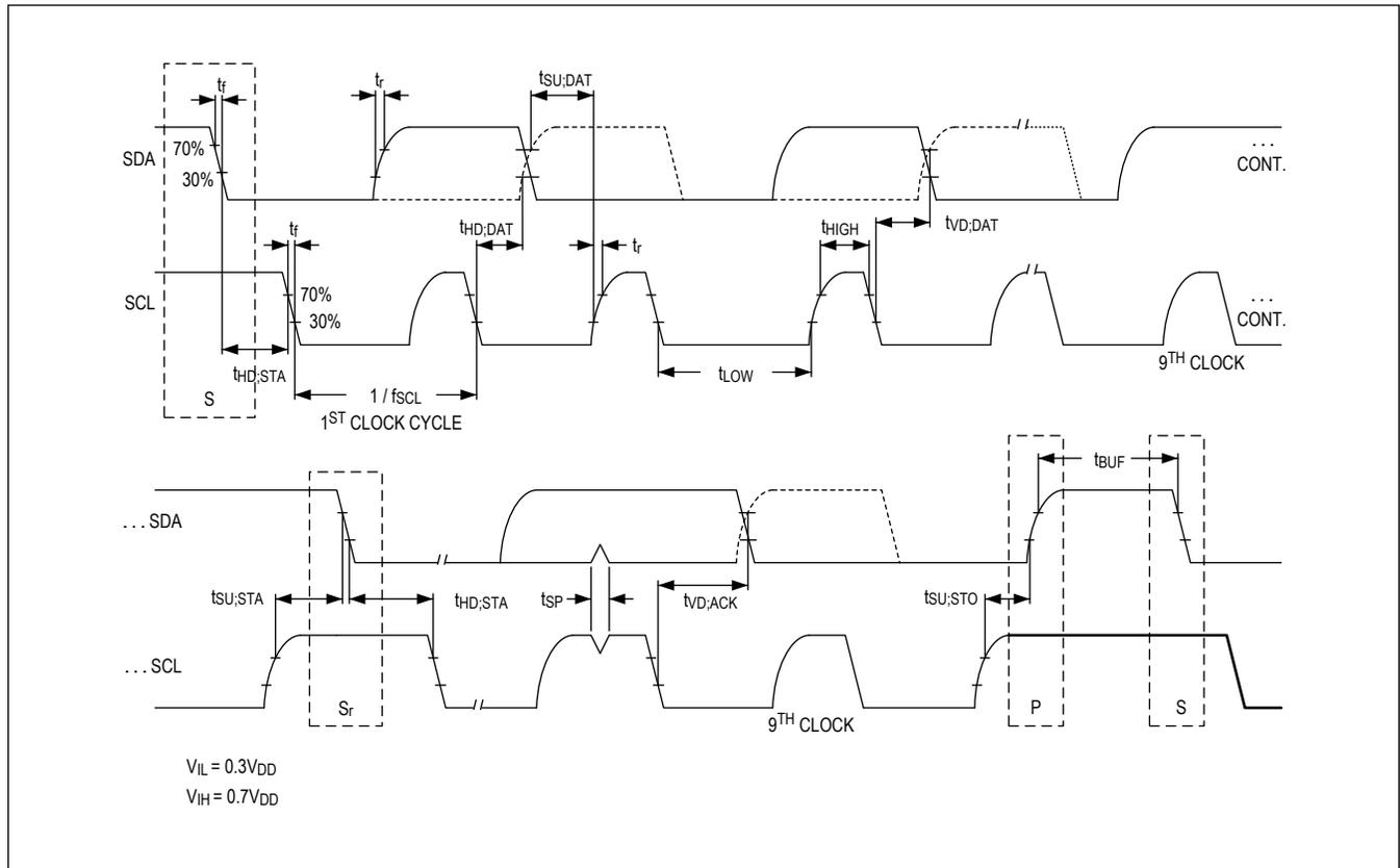
Figure 74. Standard I<sup>2</sup>C BUS Timing Diagram
