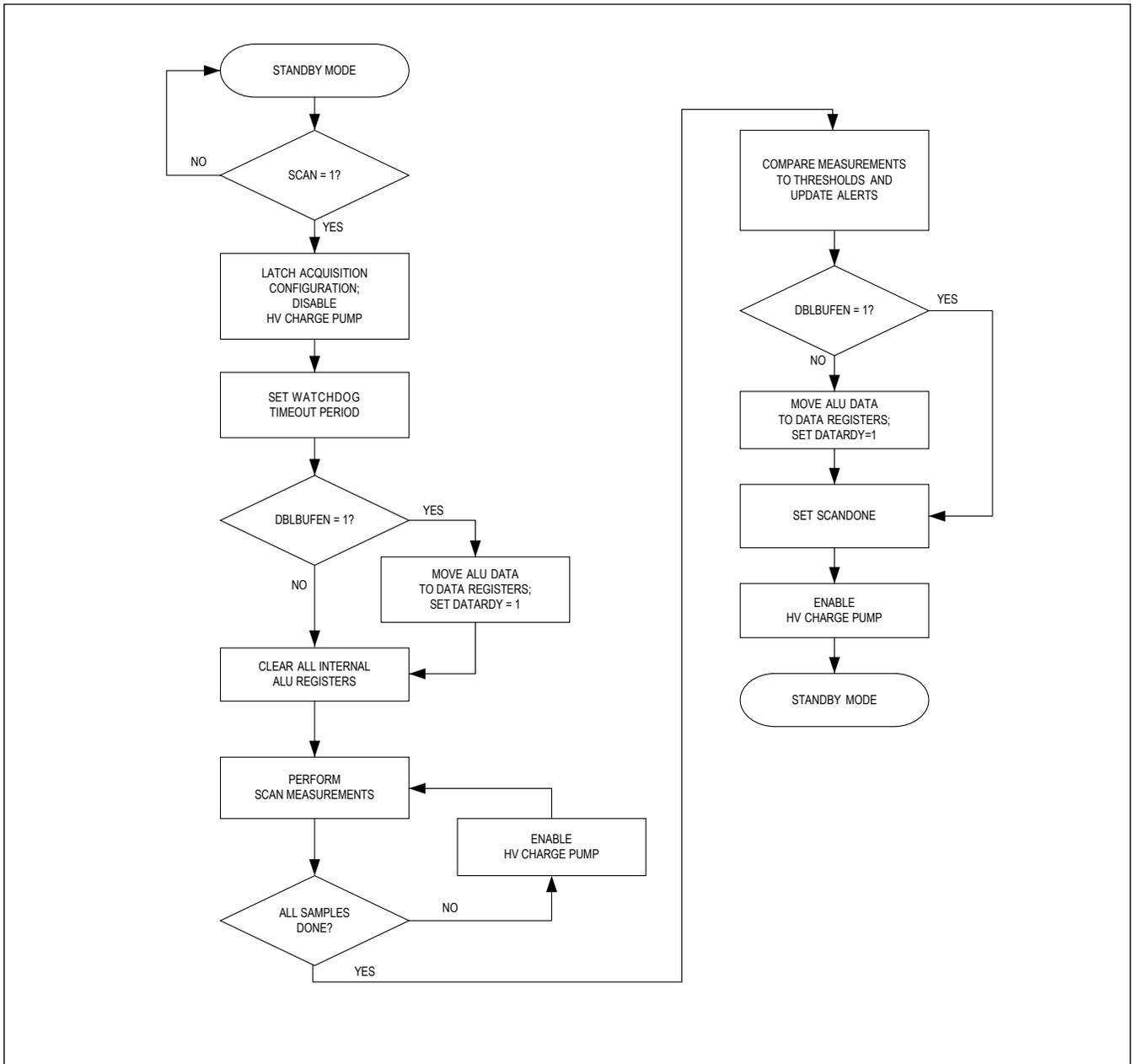
Figure 36. Acquisition-Mode Flowchart
