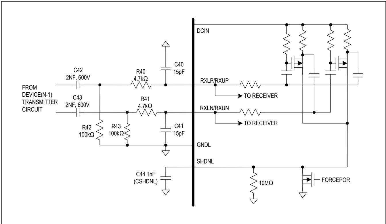
Figure 62. SHDNL Charge Pump
