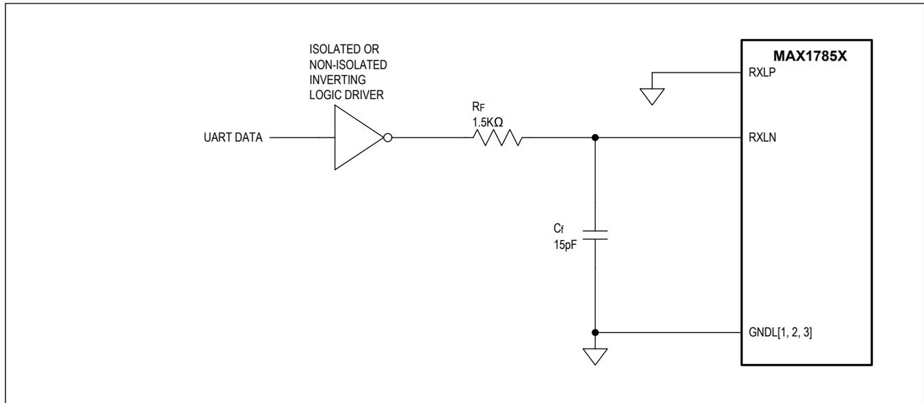
Figure 123. Application Circuit for Single-Ended UART Mode
