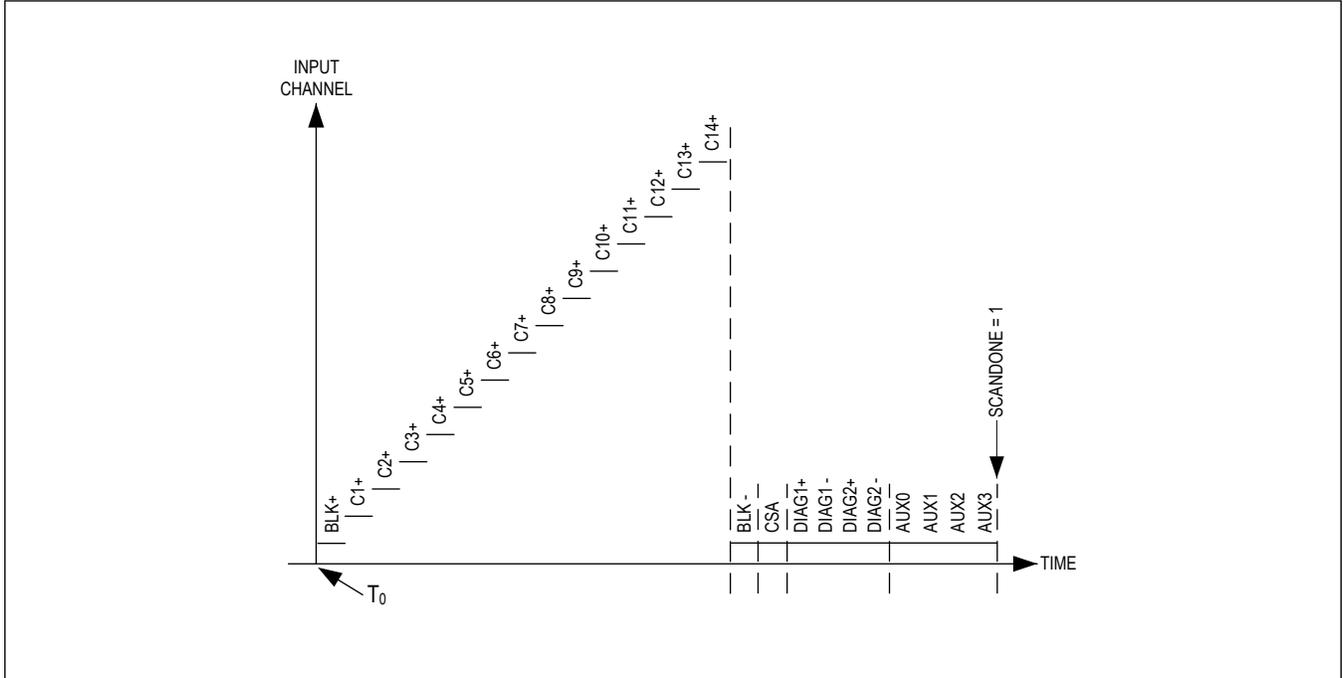
Figure 27. Acquisition - SCANCFG = 0h, SCANMODE = 1, OVSAMPL = 0h, ALTMUXSEL = 0, BLOCKEN = 1, CSAEN = 1
