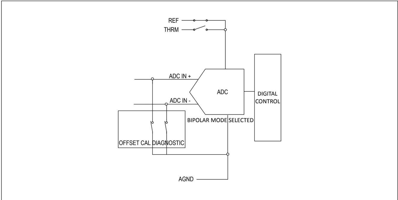
Figure 96. Offset-Calibration Diagnostic
