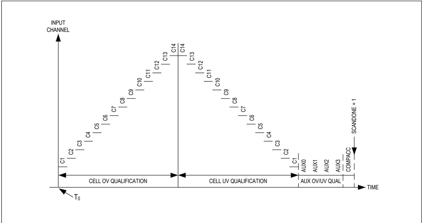
Figure 94. Comparator Accuracy End of Scan Measurement
