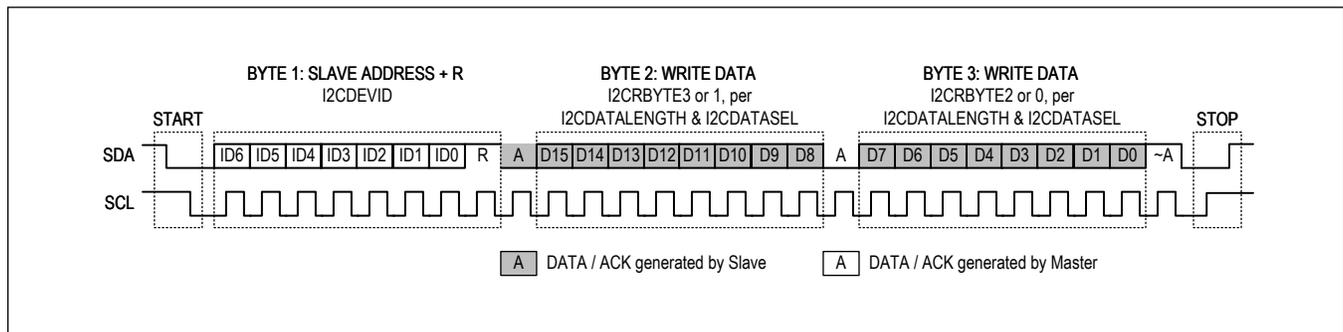
Figure 82. I<sup>2</sup>C Normal Format Read Mode Transaction Example -- 7-Bit Address, I2C10BIT = 0, I2CRFMT = 0
