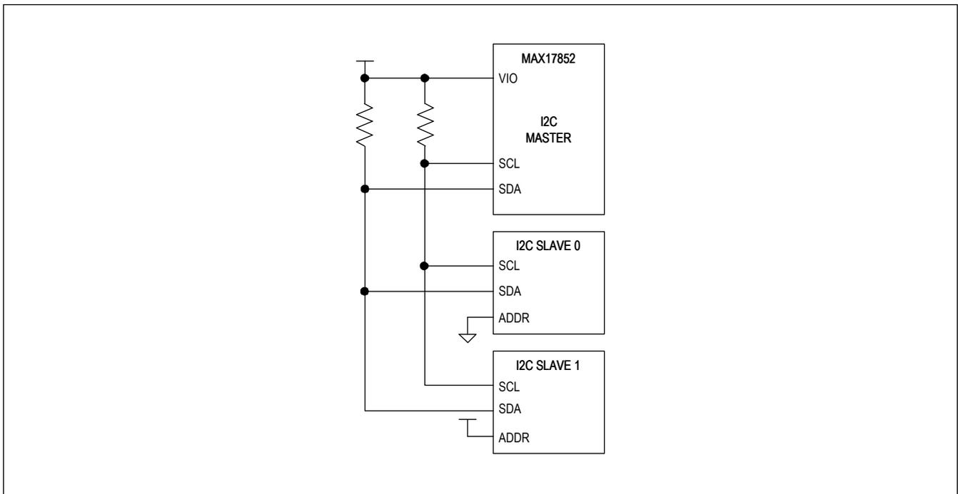
Figure 75. I<sup>2</sup>C Device Connection
