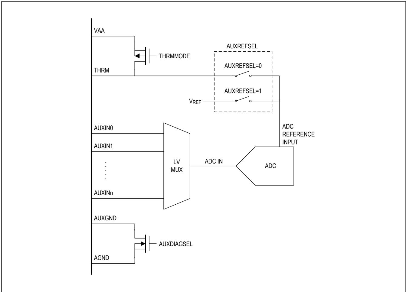
Figure 10. Auxiliary-Temperature Measurements
