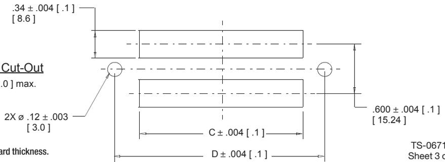
Note: Plated-through mounting holes for .062 [1.57] board thickness.
