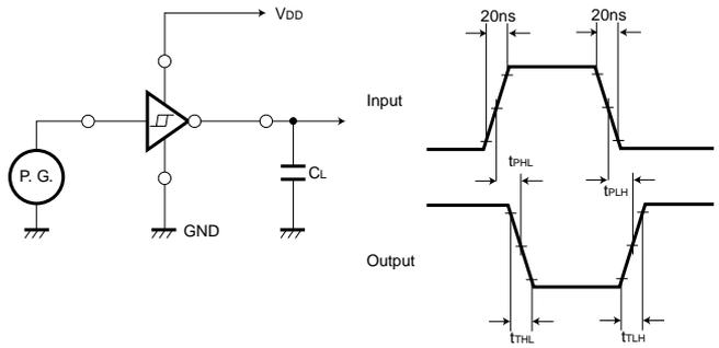
Fig.2 Switching characteristics
