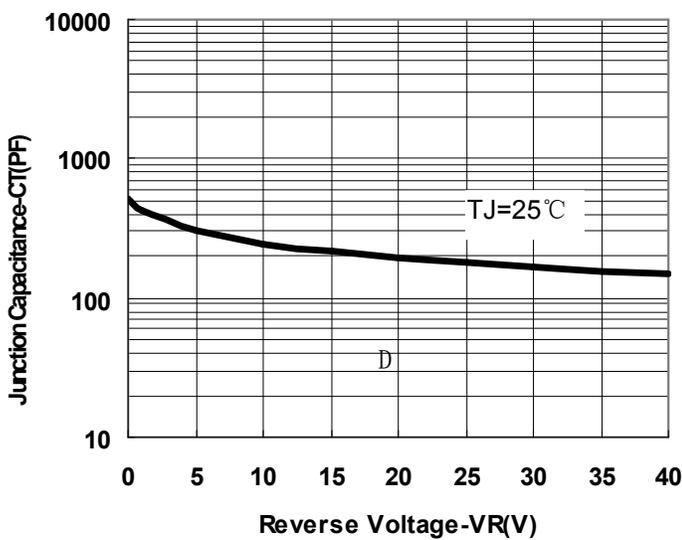
Fig.1-Typical Junction Capacitance
