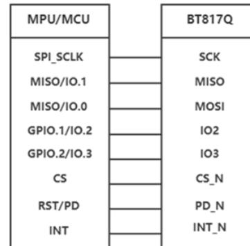
**SPI Interface** – the SPI slave interface operates up to 30MHz.
