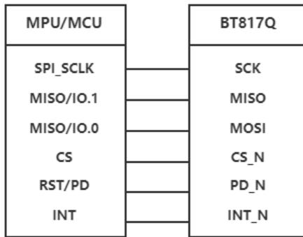
Figure 6. QSPI interface connection
