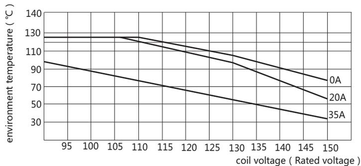
instruction : when the relay coil is applied to the maximum continuous operating voltage,the contact should not be loaded
