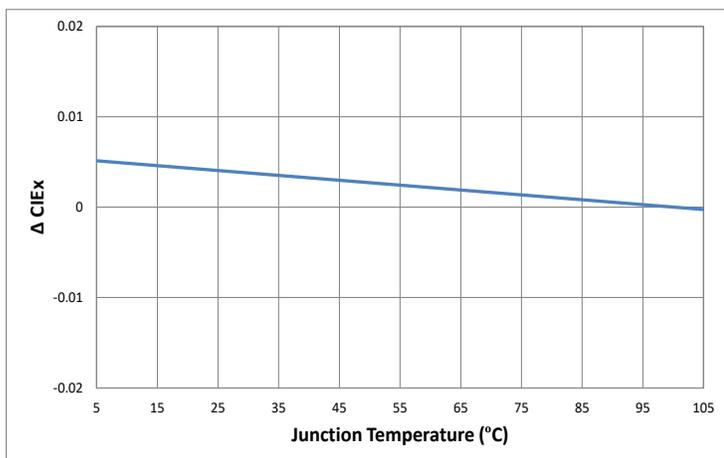
**Change in CIE<sub>y</sub> vs. Junction Temperature (3100K)**
