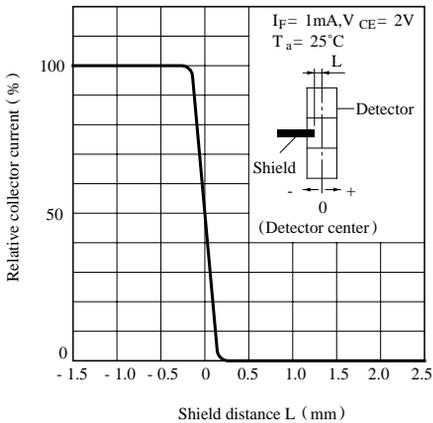
**Fig. 13 Relative Collector Current vs. Shield Distance (2)**
