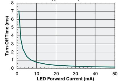
Typical  $I_F$  for Switch Operation
