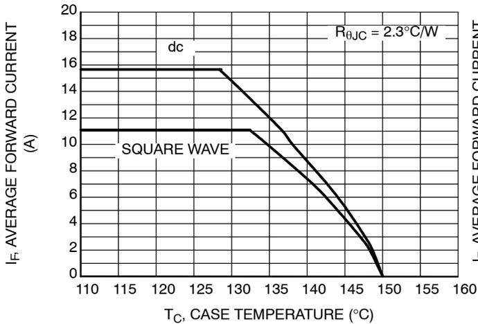
Figure 5. Current Derating, Case per Leg
