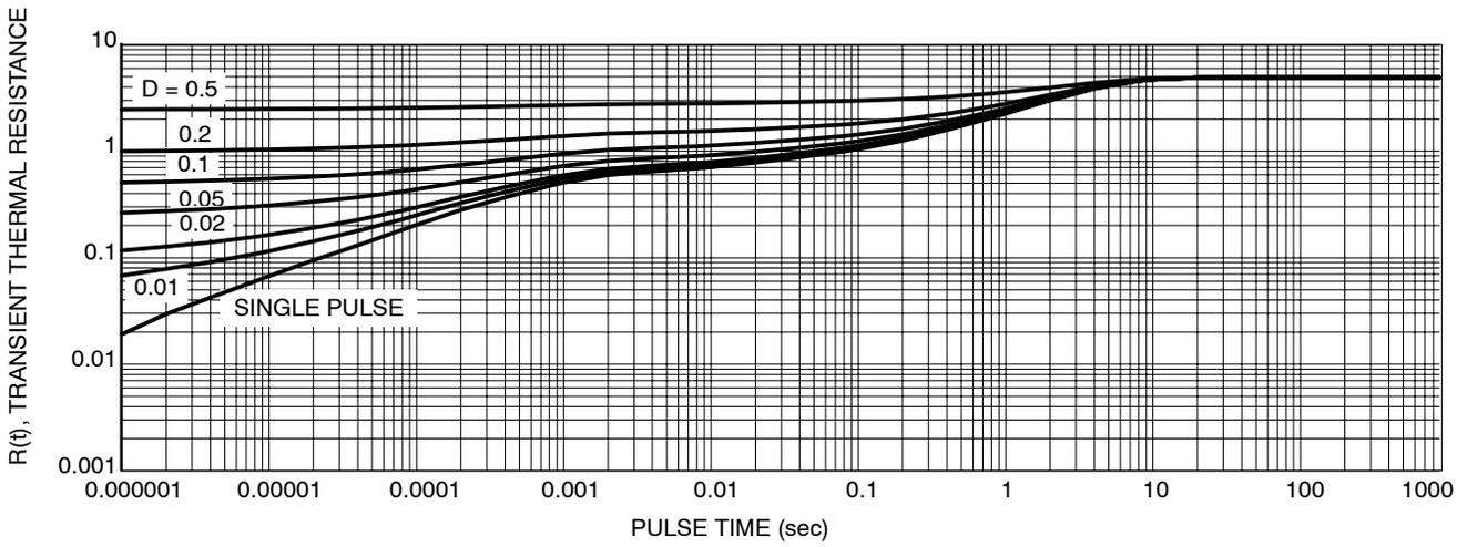
Figure 13. Thermal Response Junction-to-Case, per Leg for MBRF20L60CT
