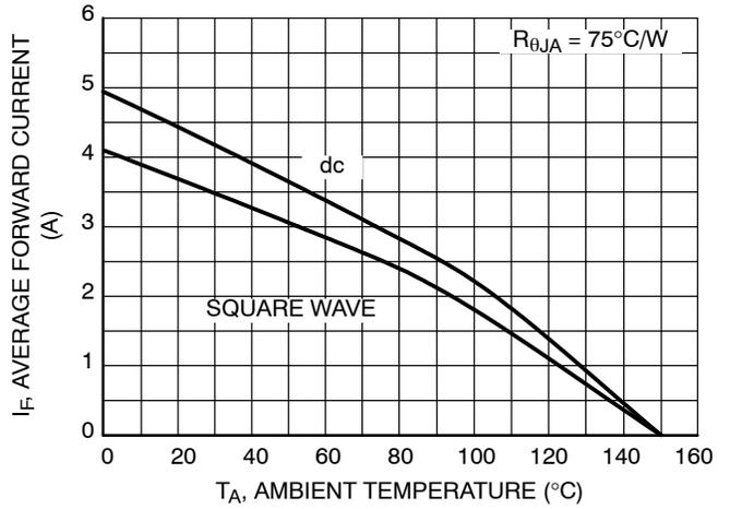
**Figure 8. Current Derating, Ambient per Leg
