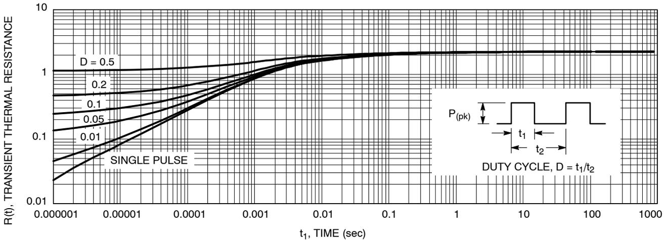
**Figure 11. Thermal Response Junction-to-Case, per Leg for MBR20L60CT**
