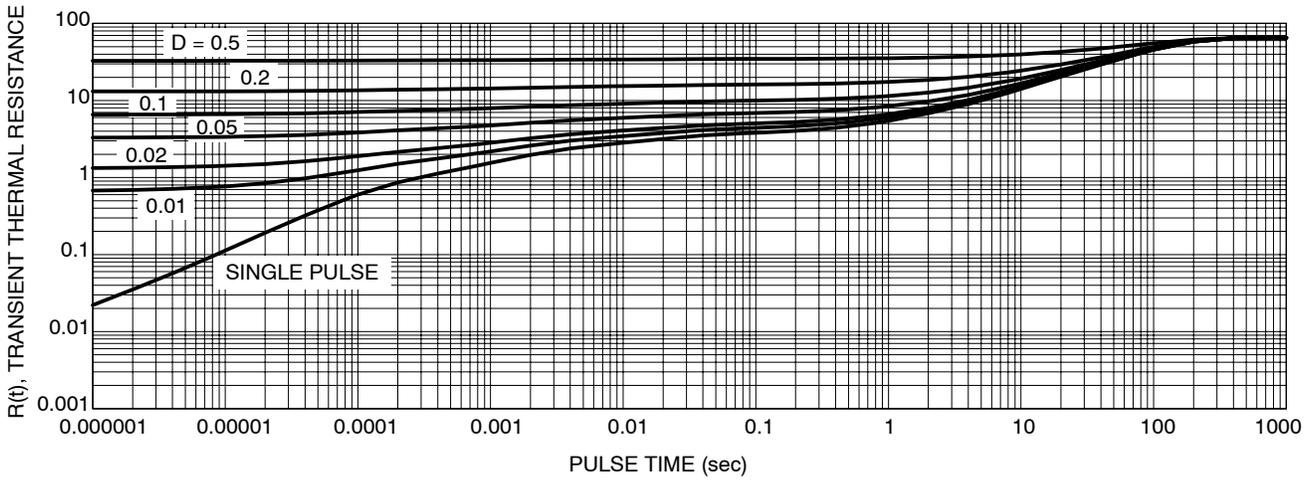
Figure 12. Thermal Response Junction-to-Ambient, per Leg for MBR20L60CT
