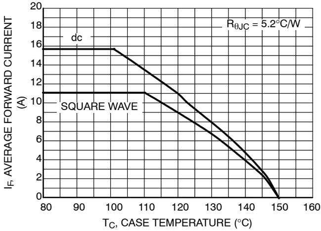
**Figure 7. Current Derating, Case per Leg
