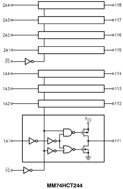
Figure 1. Logic Diagrams
