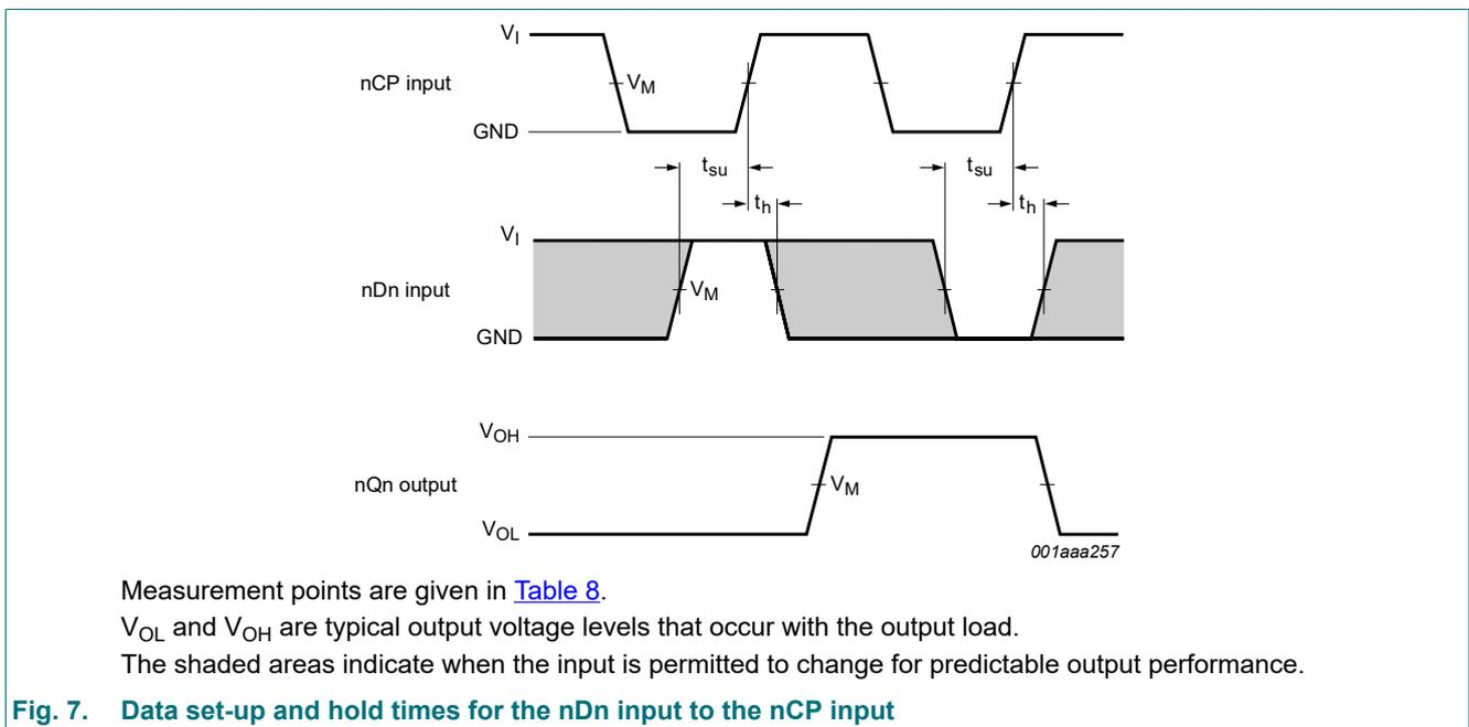
16-bit edge-triggered D-type flip-flop with 30 Ω series termination resistors; 5 V input/output tolerant; 3-state
