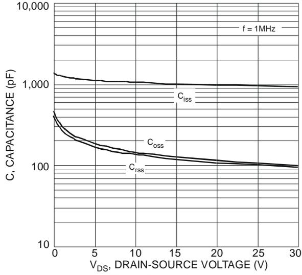
Fig. 20 Typical Capacitance
