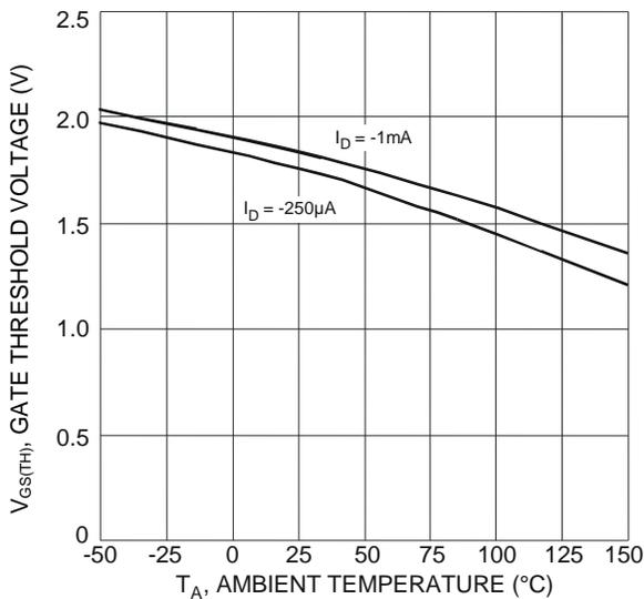
Fig. 18 Gate Threshold Variation vs. Ambient Temperature
