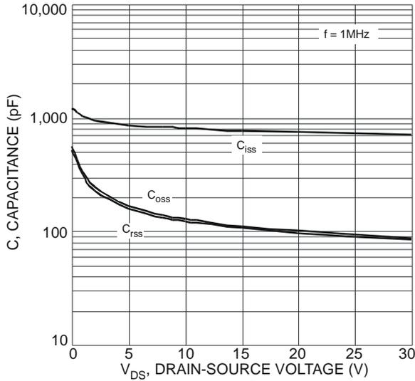
Fig. 9 Typical Capacitance
