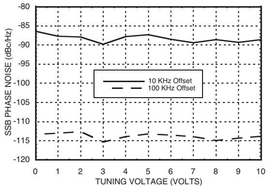
**Typical SSB Phase Noise @  $V_{tune} = +5V$**
