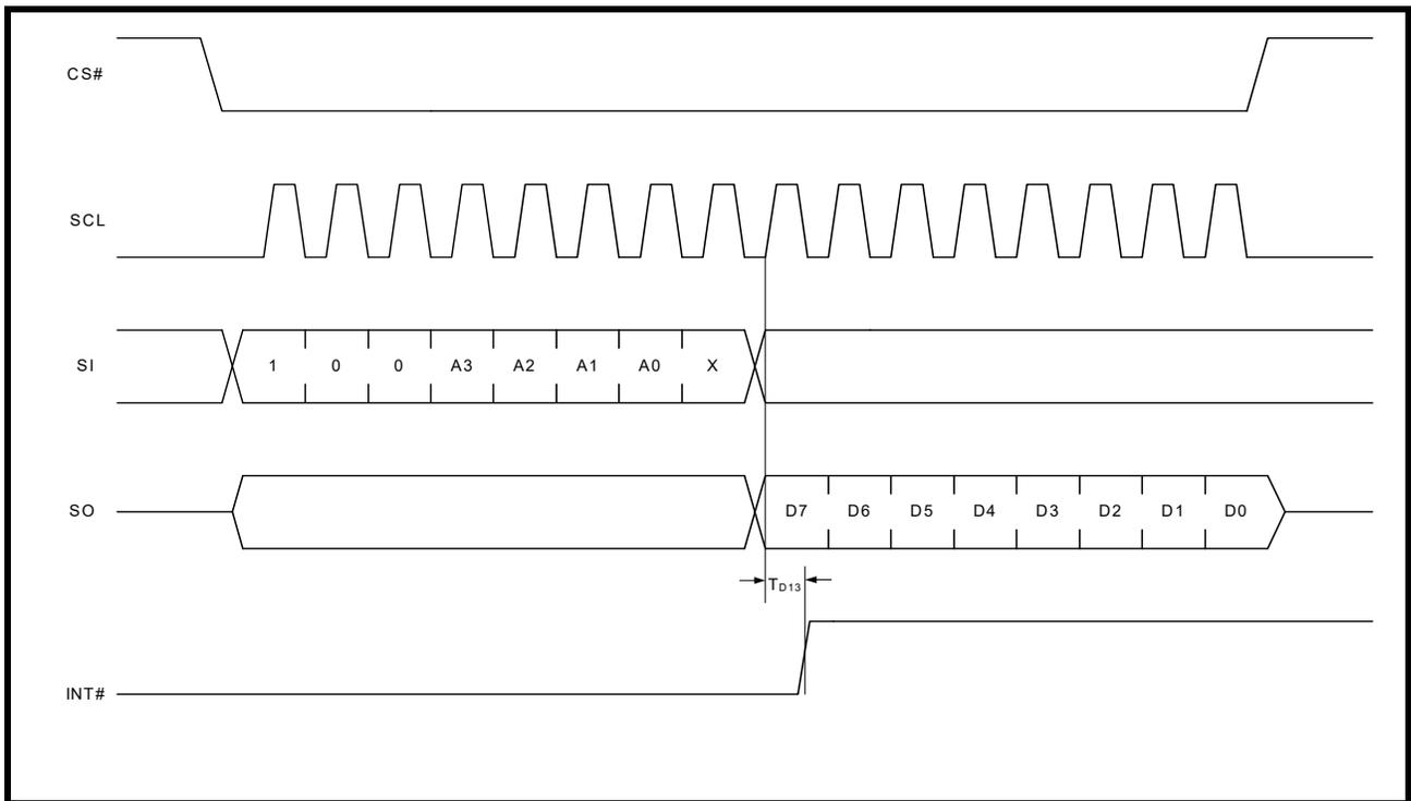
FIGURE 7. SPI WRITE OUT TO GPIO SWITCH
