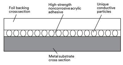
Figure 2 Embossed Backing with "Through-the-Adhesive" Contact
