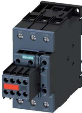
Contactor, AC-3, 30 kW / 400 V, 2 NO + 2 NC, 110 V AC, 50 Hz, 120 V, 60 Hz, with inserted varistor, 3-pole, Size S2, screw terminal Captive auxiliary switch
