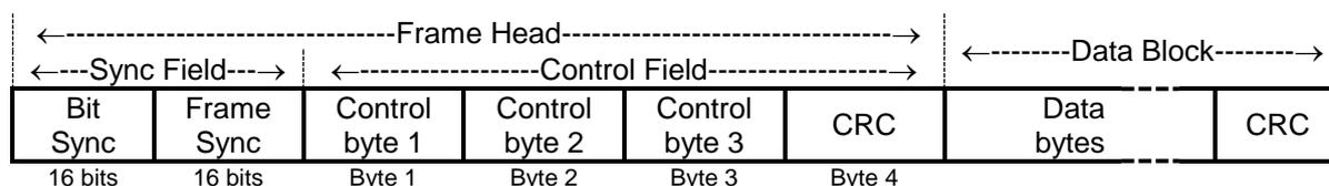
**Figure 15 Formatted Data Over Air Signal Format**
