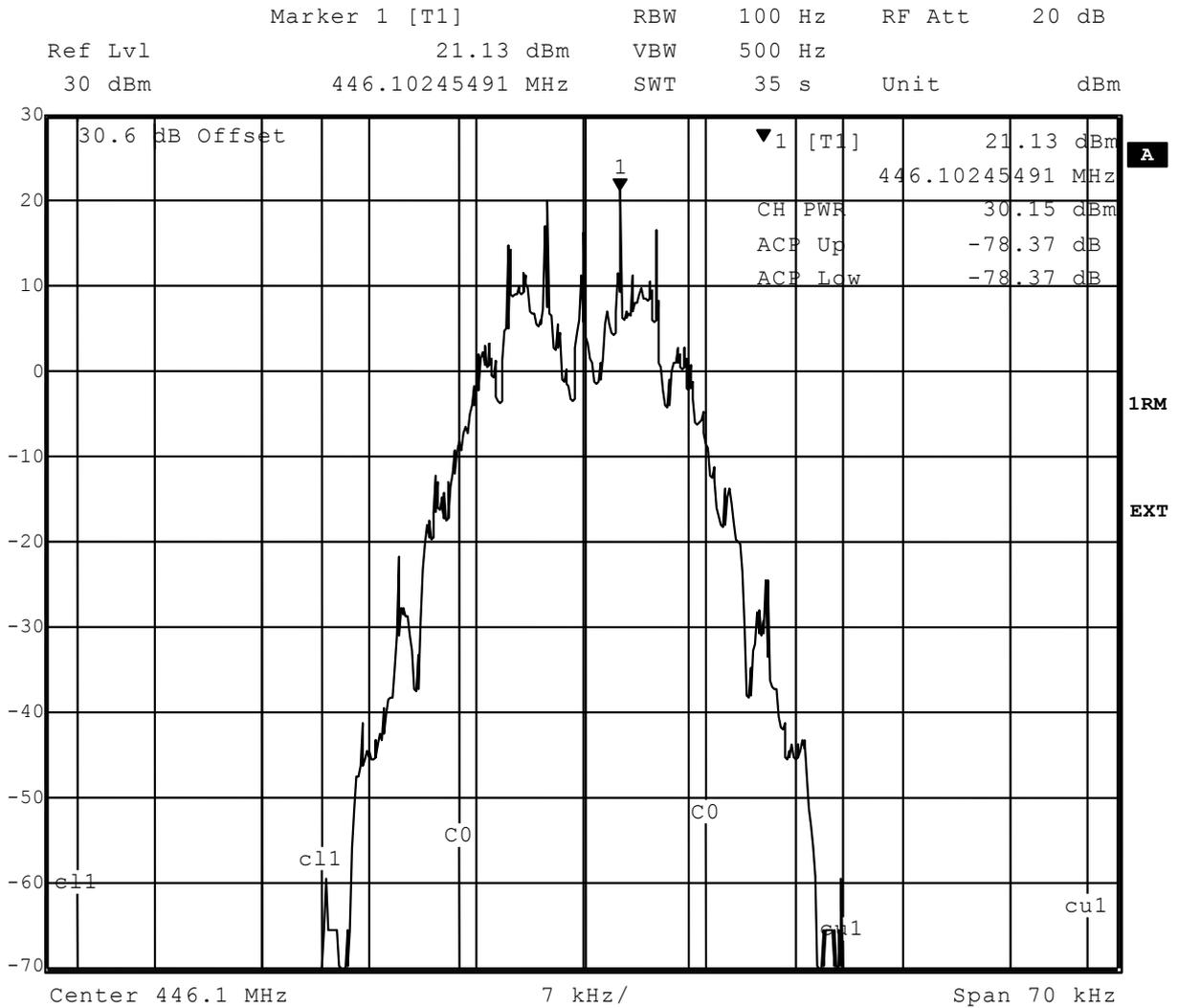
**Figure 16 Tx Modulation Spectra (FFSK/MSK) - 2400bps, 5kHz deviation**
