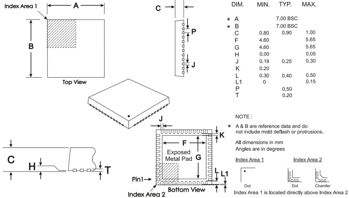
Depending on the method of lead termination at the edge of the package, pull back (L1) may be present.
