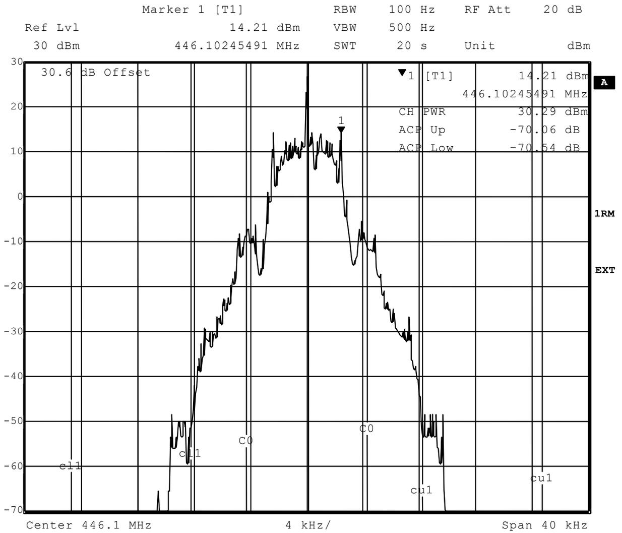
**Figure 17 Tx Modulation Spectra (FFSK/MSK) - 2400bps, 1.5kHz deviation**
