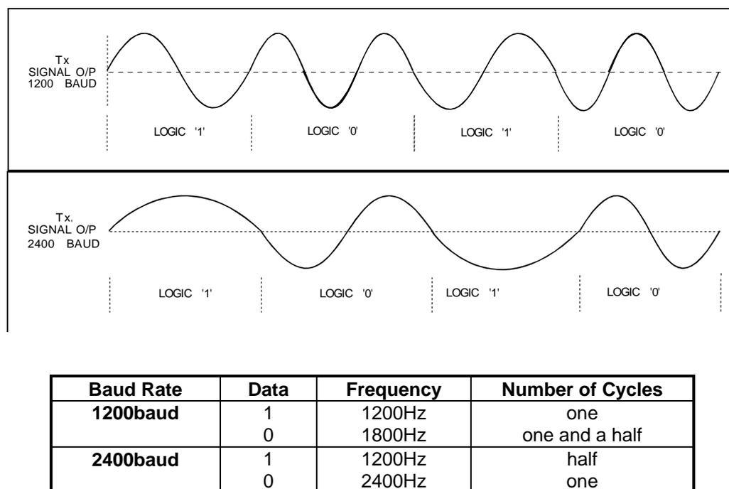
**Figure 13 Modulating Waveforms for 1200 and 2400 Baud MSK/FFSK Signals**
