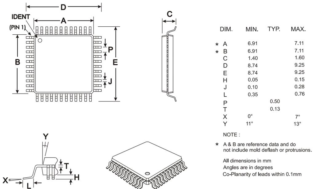
**Figure 20 Mechanical Outline of 48-pin LQFP (L4)**
