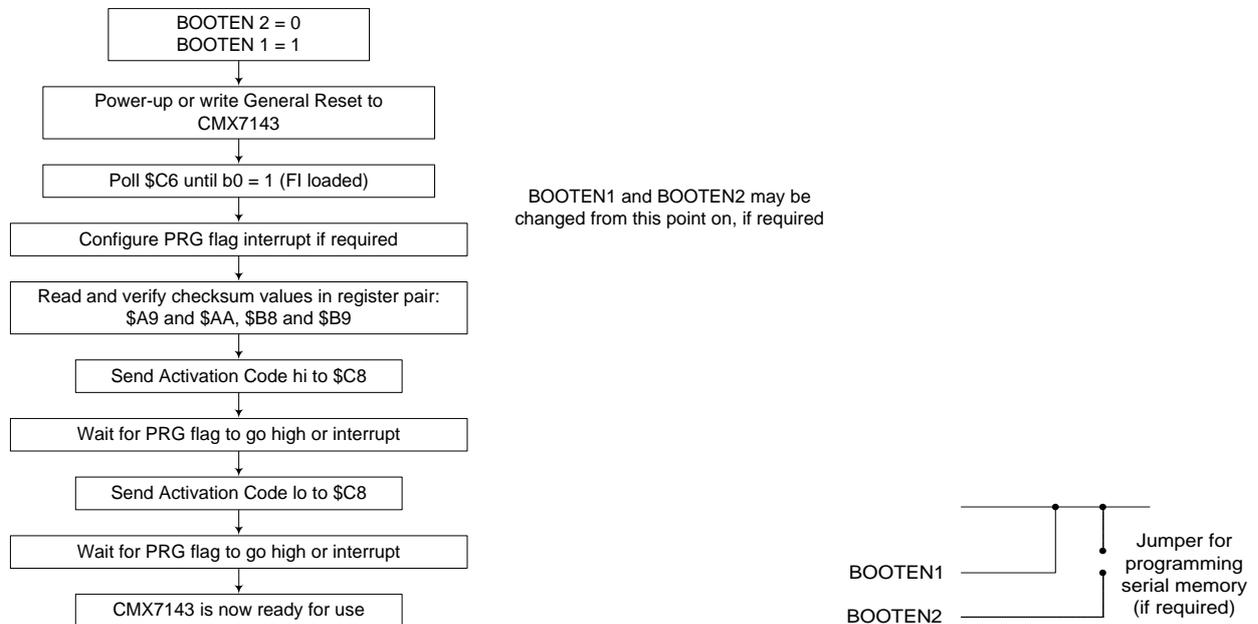
Figure 6 FI Loading from Serial Memory
