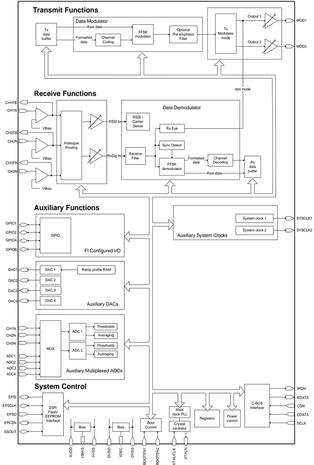
Figure 1 Block Diagram
