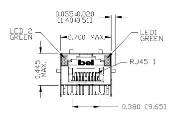
0,125 [3,17] SIGNAL & LED LEADS 0,051 [1,30] MIN [3,81] | LEADS ├<del>-</del> 0,950 MAX. --0,150 CGROUND 0.100 [2.54] 0.100 [2.54] PITCH 0,360 [9,14] 0.350 [8.89]
