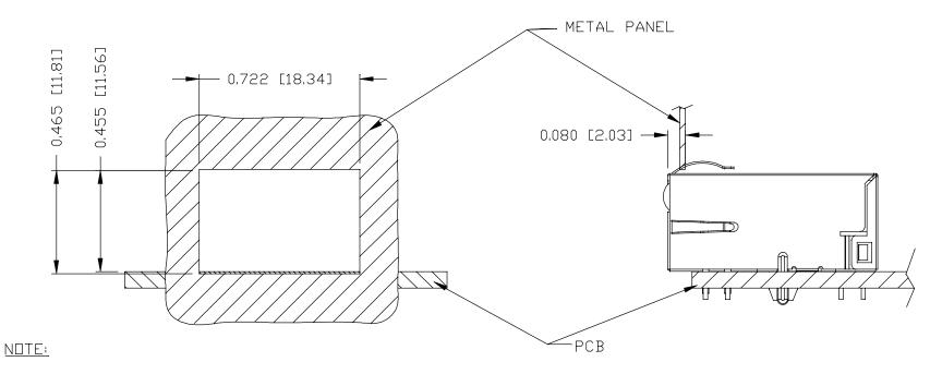
THE DISTANCE OF PANEL INSIDE SURFACE RELATIVE TO FRONT SURFACE OF PART IS ONLY A SUGGESTION. IN CASE THIS DISTANCE IS DIFFERENT, THE REQUIRED PANEL OPENING DIMENSIONS CHANGE ACCORDINGLY.
