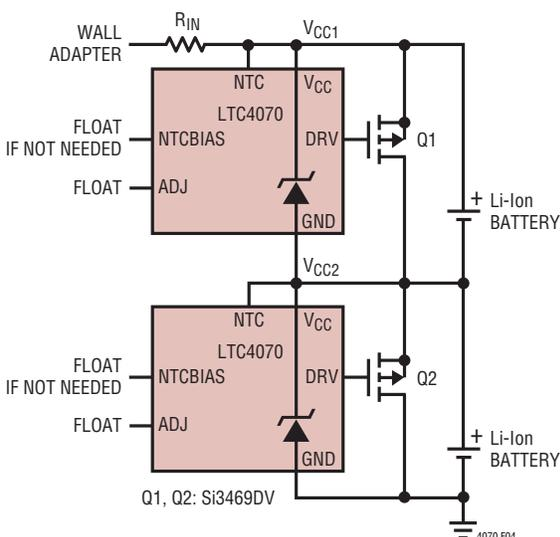
Figure 4. 2-Cell Battery Charger with Boosted Drive
