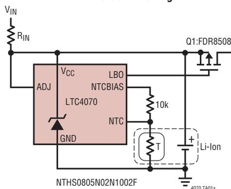
**NTC Overtemperature Battery Float Voltage Qualifying**
