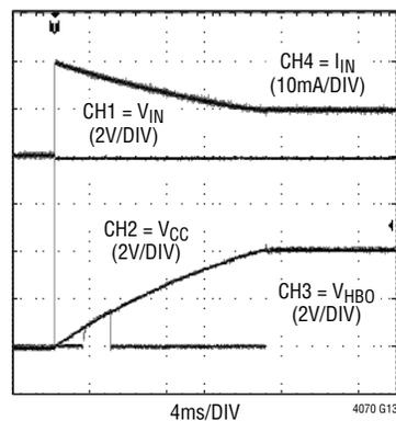
**Step Response with 800mAHr Battery,  $R_{IN} = 81\Omega$**
