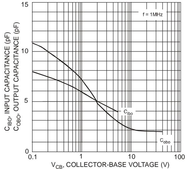
Fig. 2, Input and Output Capacitance vs. Collector-Base Voltage
