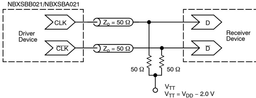
**Figure 4. Typical Termination for Output Driver and Device Evaluation**
