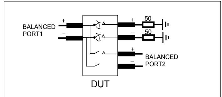
**Differential Off Isolation Test Circuit**
