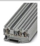
Feed-through terminal block, Connection method: Spring-cage connection, Cross section: 0.08 mm² - 6 mm², AWG: 28 - 10, Width: 6.2 mm, Color: yellow, Mounting type: NS 35/7,5, NS 35/15
