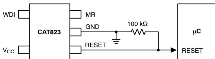
Figure 11.  $\overline{\text{RESET}}$  Valid to 0 Volts  $V_{\text{CC}}$
