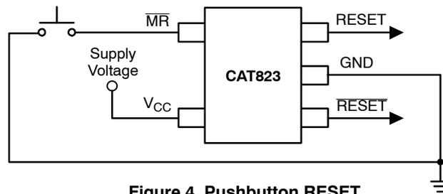
Figure 4. Pushbutton RESET
