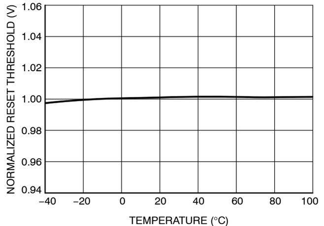
**Figure 3. Normalized Reset Threshold Voltage vs. Temperature**
