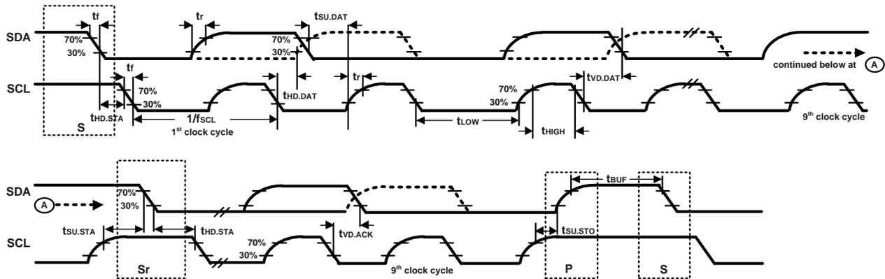
**Figure 1. I<sup>2</sup>C Bus Timing Diagram**
