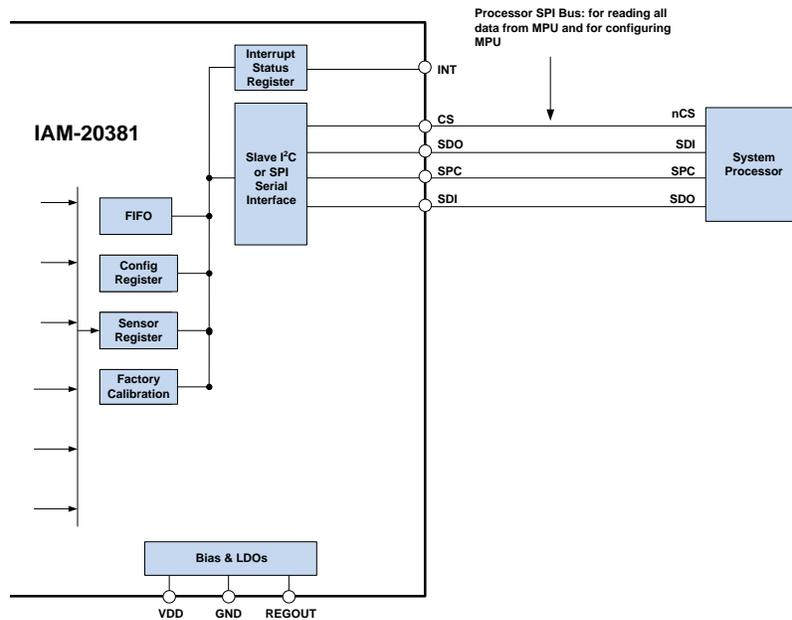
**Figure 7. IAM-20381 Solution Using SPI Interface**
