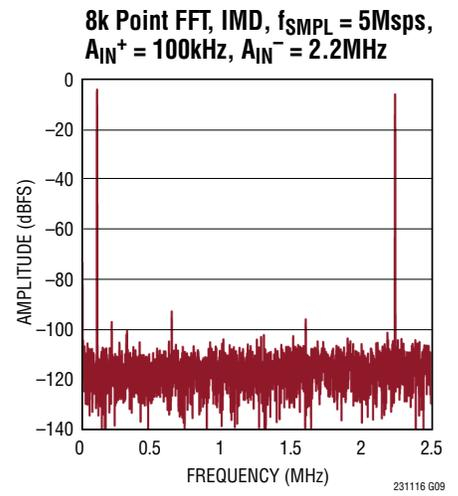
**TYPICAL PERFORMANCE CHARACTERISTICS**  $T_A = 25^\circ\text{C}$ ,  $V_{DD} = 5\text{V}$ ,  $OV_{DD} = 2.5\text{V}$ ,  $REF_{OUT} = 4.096\text{V}$ ,  $f_{SAMPL} = 5\text{Msps}$ , unless otherwise noted.
