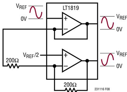
Figure 8. Single-Ended to Differential Driver
