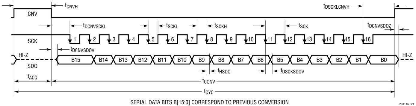
Figure 21. LTC2311-16 Timing Diagram, CMOS, LVDS I/O Modes
