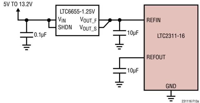
Figure 13a. LTC2311-16 with an External REFIN Voltage
