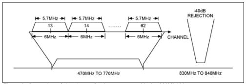
Figure 2. Illustration of the channelization process with the MAX2160 tuner.
