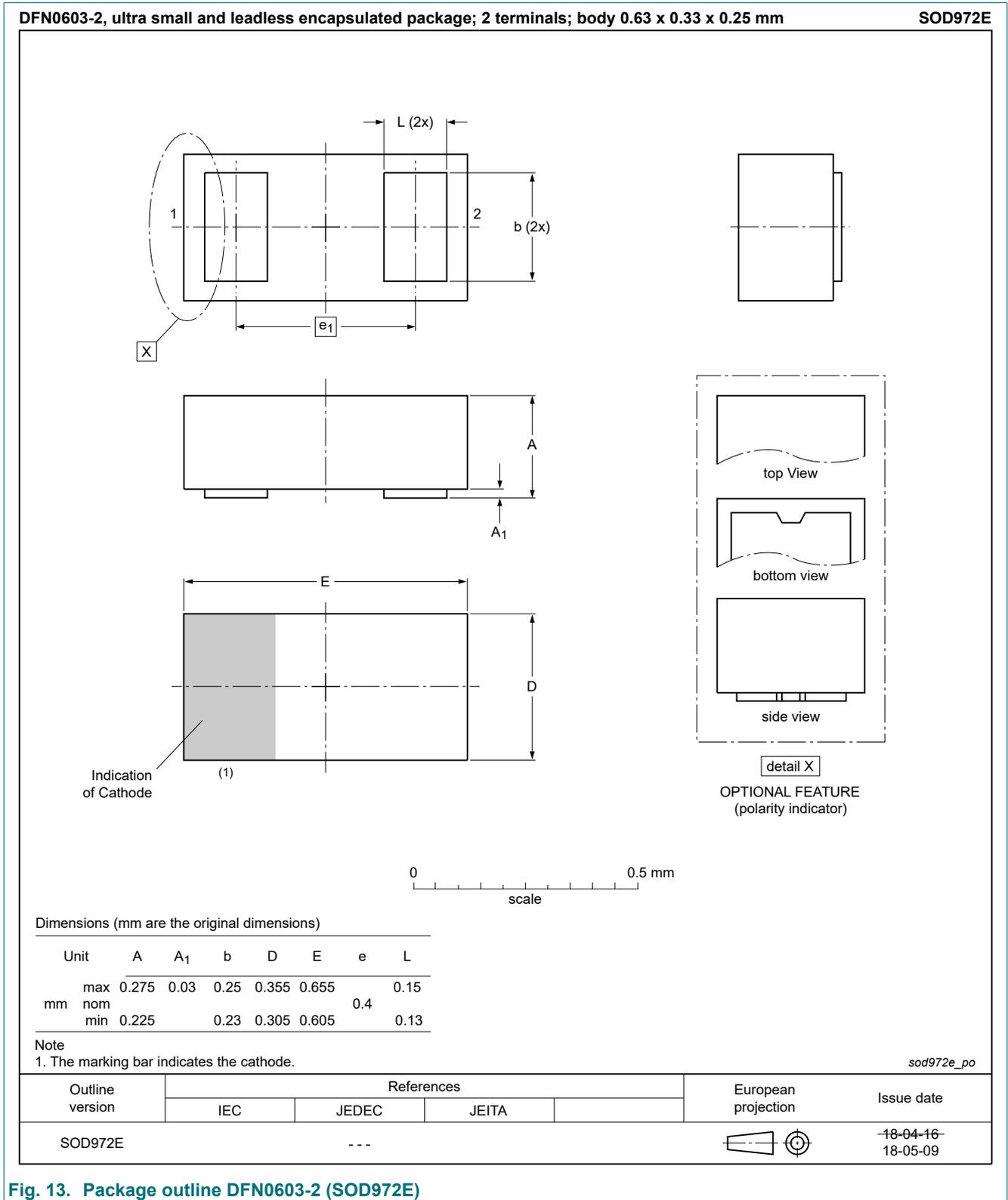
Fig. 13. Package outline DFN0603-2 (SOD972E)
