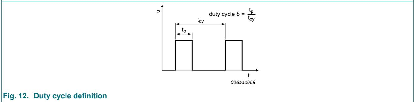
Fig. 12. Duty cycle definition
