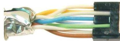
Slide load bar to end of pairs to make loading into housing easier
