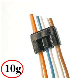
Insert Org Blu and Brn pairs into load bar
