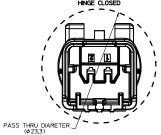
1 MM ADDITIONAL CLEARANCE ADDED TO TIGHTEST FIT CIRCLE 2 WAY MALE WITH FORD CLIP SLOT
