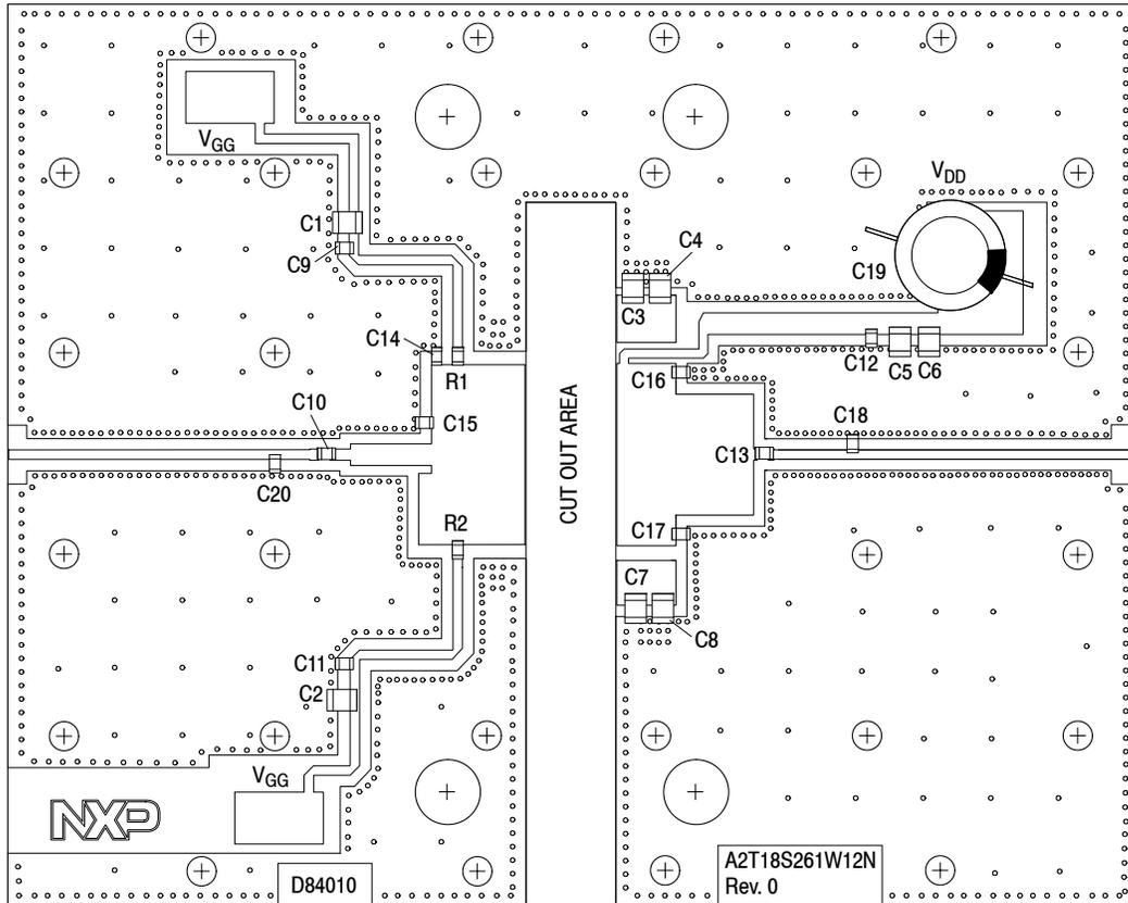
Figure 2. A2T18S261W12NR3 Test Circuit Component Layout
