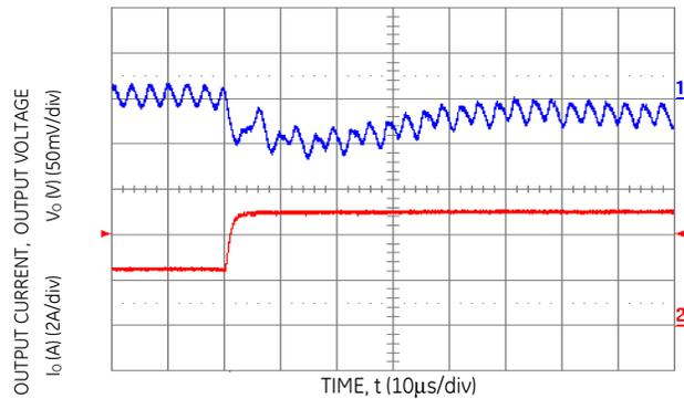
**Figure 13. Transient Response to Dynamic Load Change from 50% to 100% of full load (Vo = 5.0 Vdc, Cext = 2x150 µF Polymer Capacitors).**
