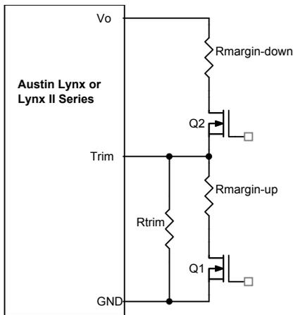
Figure 33. Circuit Configuration for margining Output voltage.
