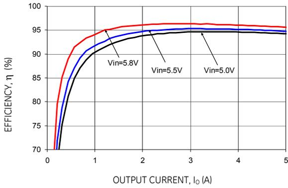
Figure 7. Converter Efficiency versus Output Current ( $V_{out} = 4.0Vdc$ ).
