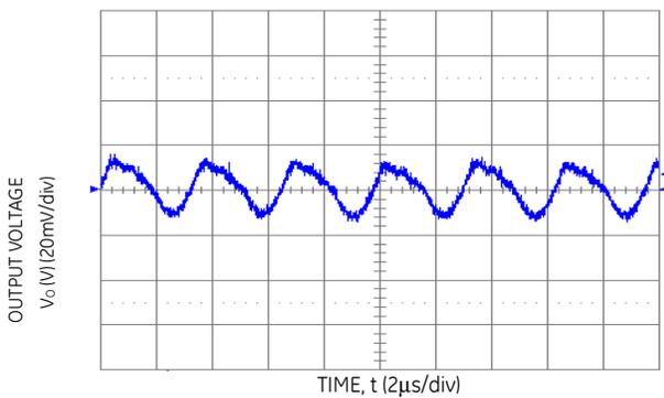
**Figure 10. Typical Output Ripple and Noise**
