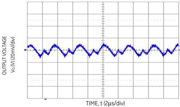
**Figure 9. Typical Output Ripple and Noise**
