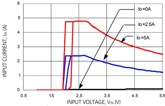
**Figure 8. Input voltage vs. Input Current**
