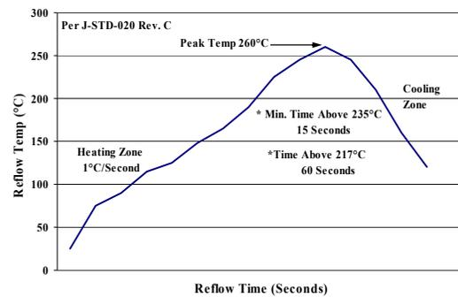
Figure 38. Recommended linear reflow profile using Sn/Ag/Cu solder.
